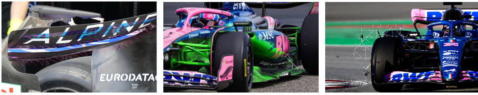
Figure 1.2: Flow measurement devices for on-site full-scale testing of a race car. Left: tufts fitted on the rear wing. Middle: oil-flow visualization of the front suspension arms. Right: pressure rake on the front tyre wake.
