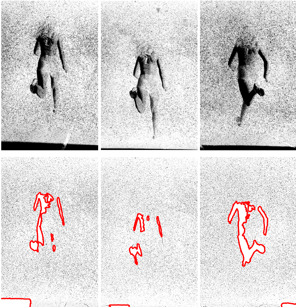
Figure 4.14: Experimental images of the flow in the near wake of a running athlete. Images from cameras 1a to 1c (see figure 4.13) given from left to right. Top: raw images. Bottom: pre-processed images (spatio-temporal high-pass filter), with masked regions indicated in red.
