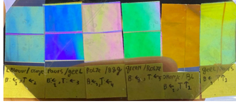
Figure 3.8: A snapshot of several different tape orientations viewed through the secondary polariser.
