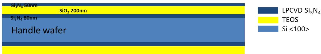
**Fig. 4-17** At the end of Step 1. The Si wafer is deposited with TEOS and Si<sub>3</sub>N<sub>4</sub> thin films.
