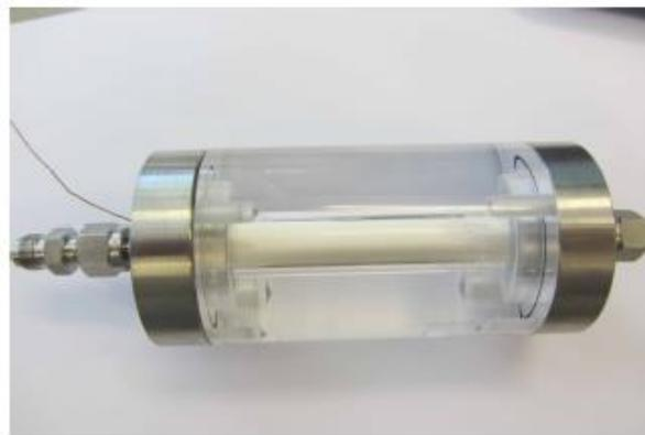
**Fig. 6-12** High voltage gas feedthrough test structure built for testing the concept described in Fig. 6-11. The diode structure is made of plexiglass is about 9 cm long and filled with alumina beads (1-100 µm in diameter) inside. The structure showed no gas discharge breakdown in the gas pressure range 1 mbar to 1 bar while high voltage up to 30 kV was applied. The test gases were helium, nitrogen, and argon.
