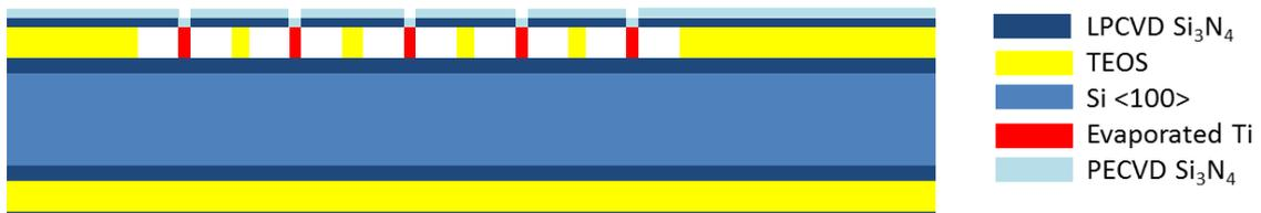
**Fig. 4-22** After lifting off of the evaporated Ti from the  $\text{Si}_3\text{N}_4$  masking layer, 50 to 100 nm PECVD  $\text{Si}_3\text{N}_4$  is additionally evaporated to completely close the etch access holes.
