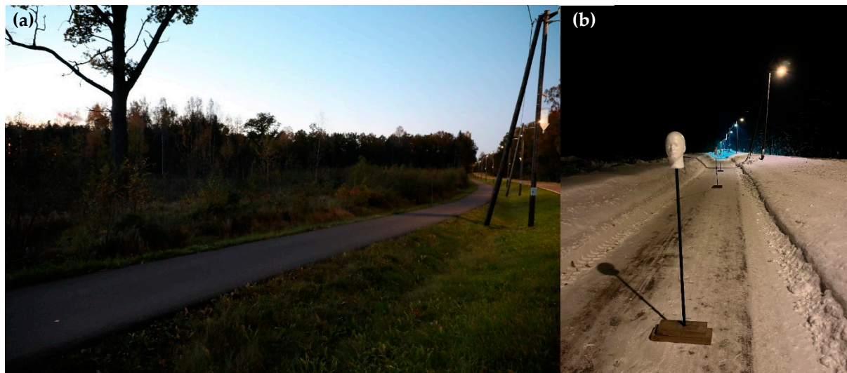
Figure 1. Image (a) shows the footpath with the clear-cut area on its left and the road on its right, with luminaires positioned between the road and the footpath. Image (b) shows the head-shaped light probe in one of the luminaire groups and in snowy conditions.
