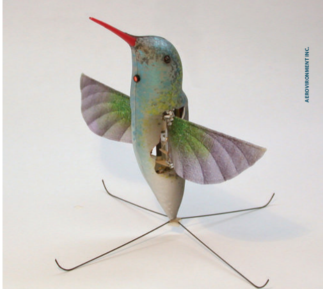
Figure 2. Demonstration of the drone by Matthew Keennon, the hummingbird UAV Project manager
