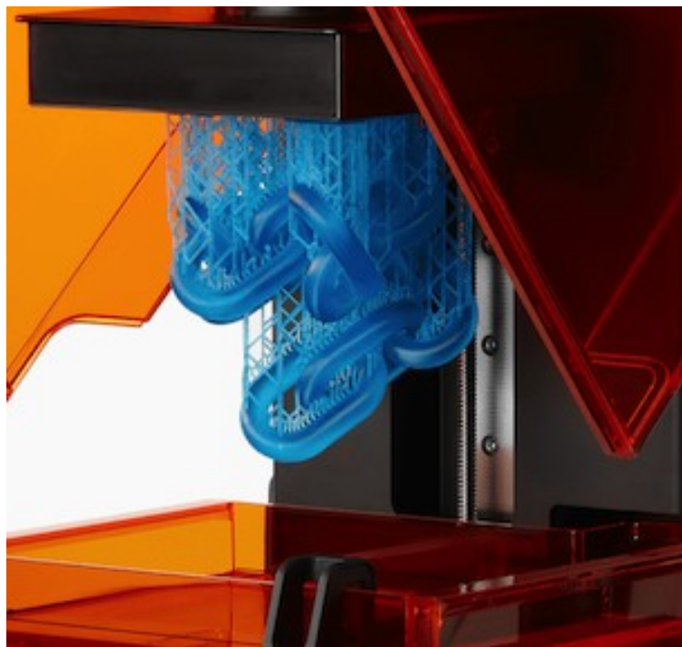
Figure 9, Object printed with SLA-bottom, with support structures. [20]
