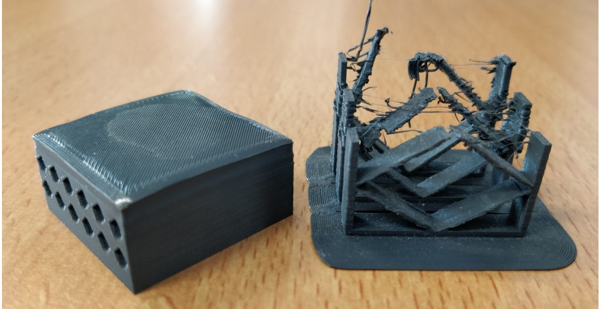
Figure 16, Photograph of two unsuccessful test prints using the Ultimaker3 printer.
