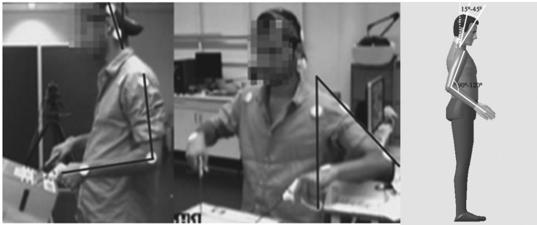
Figure 2.5 Measurement of joint angle and optimal posture of a surgeon
