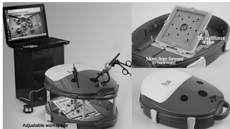
Figure 5.1 Ergo-Lap simulator: The Ergo-Lap simulator ready for use (left); the flexible arrangement of the task panel allows for ergonomic training conditions (upper right); the Ergo-Lap simulator ready for transportation (bottom right).
