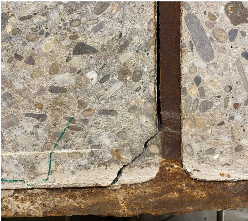
Fig.3.12. LB1. Crack at the west end of beam 1 after testing.
