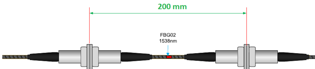
Fig.2.23. Detail of an optic fiber and an FBG sensor. (Faassen, 2021)
