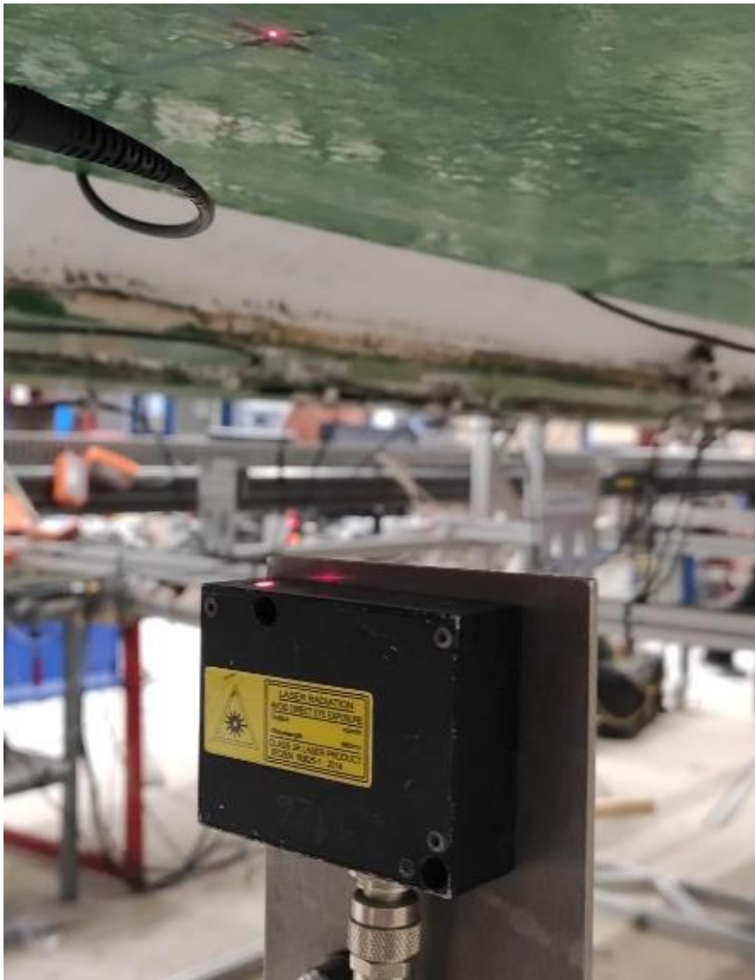
Fig.2.11. Laser measuring vertical displacement from bottom of a steel beam.
