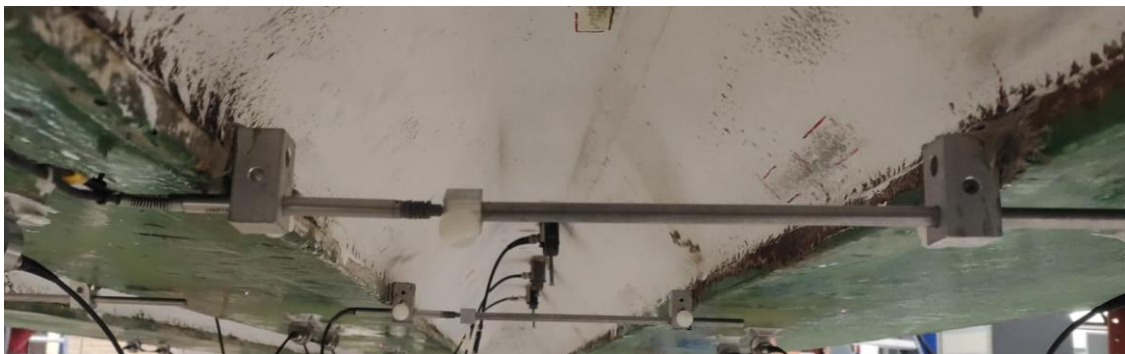
Fig.2.17. LVDT 5-10 measuring relative transverse displacement between the beams.
