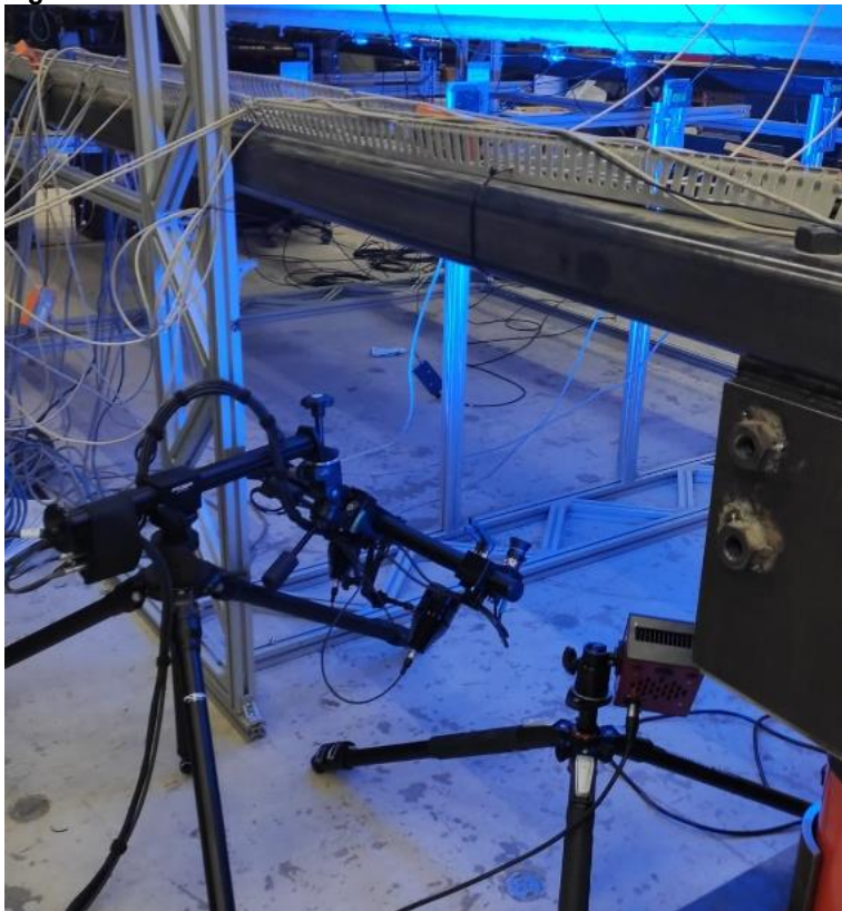
Fig.2.36. Camera and light setup 3D DIC.
