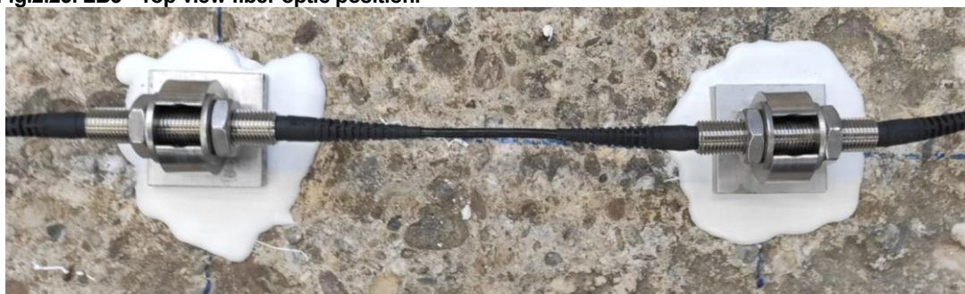
Fig.2.26. Fiber optic glued to the top of the specimen.
