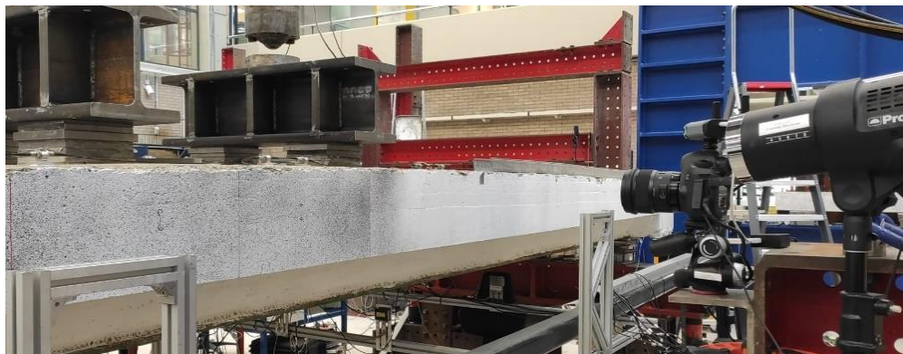
Fig.2.33. LB1 - Camera and flash setup for 2D DIC.
