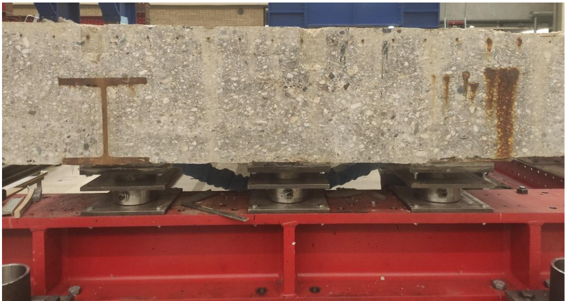
Fig.2.8. LB1 – Load Cells East view of the specimen.
