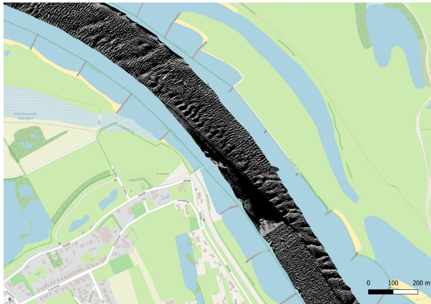
Figure 2.4: Visualization of a multibeam measurement at the end of fixed layer near St. Andries (Multibeam measurement taken at 13 March 2013)
