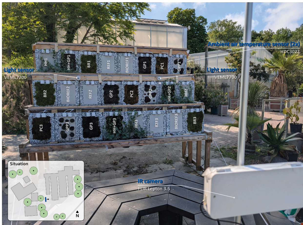
Fig. 4. Experimental set-up in the Hortus Botanicus Delft showcasing the location of the different sensors and samples.
