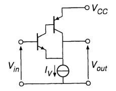
Fig. 6. A two-transistor voltage follower.
