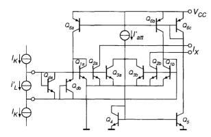
Fig. 5. A symmetrical current mirror used as a comparator. The common-mode loop gain equals two to prevent instability.
