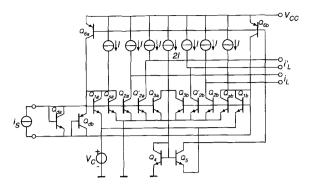
Fig. 4. A symmetrical current mirror as used in the controlled amplifier including its biasing circuitry.
