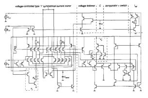
Fig. 7. The total automatic gain control. Instability may be counteracted by  $C_{\rm comp}$ .
