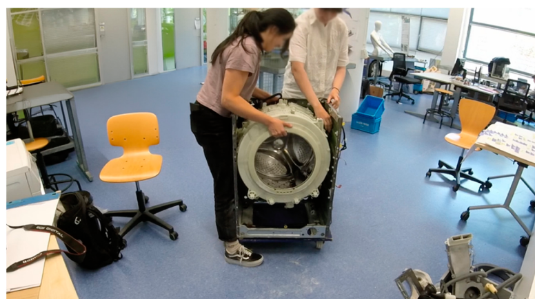
Figure 5. Disassembly of the tub requires support from an additional repairer due to its weight and fixture type. The manipulation of heavy products and components can lead to injuries if the repairer does not have help available.
