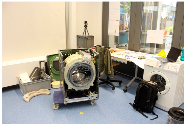
Figure 1. Experimental setup for the disassembly and reassembly of the washing machines.
