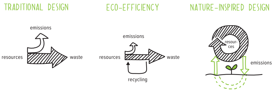
Figure 7.1: Visualisation of the differences in the primary objectives of eco-efficiency strategies and nature-inspired design strategies (NIDS) in terms of resource flows (based on Braungart et al., 2008)
