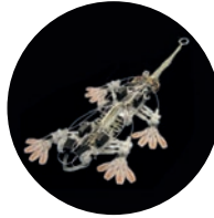
Stanford StickyBot dry adhesion climbing of vertical surfaces
