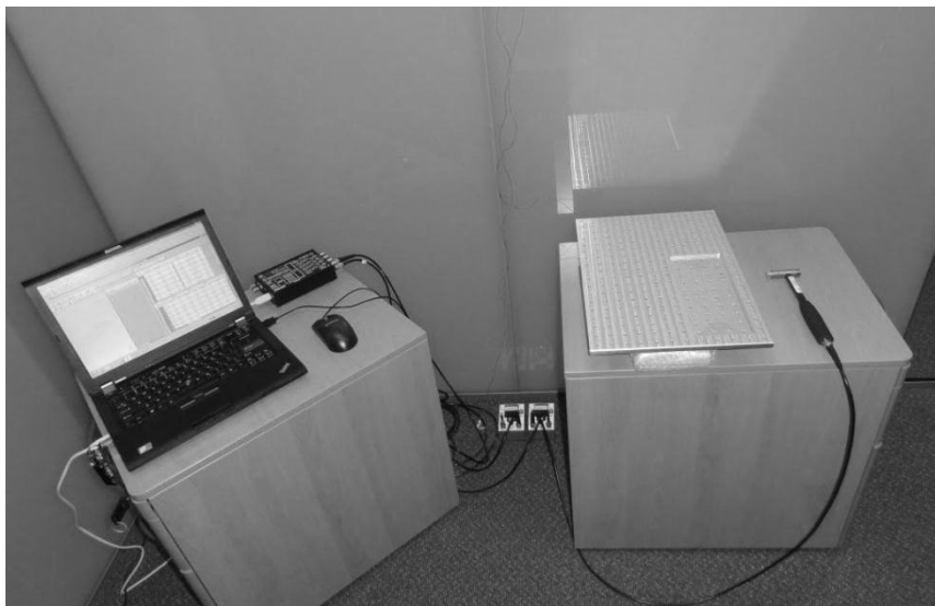
Figure 3: Experimental setup; structure, suspension (bubble foil), hammer, amplifiers, acquisition module and computer are visible. The accelerometer is not visible, since it is mounted at the bottom of the plate.
