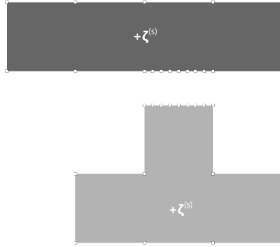
Figure 9: Reduced substructured FEM model of example structure
