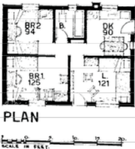
Image 7: Elevation and plan drawings of the Non-European 51/9 house, a 3 roomed house.
