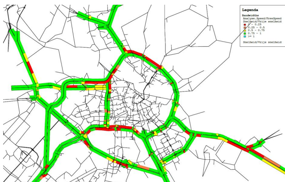
Figure 4-5. Speed/free speed plot from MARPLE at 17:30 (Retrieved on 31/10/2019)
