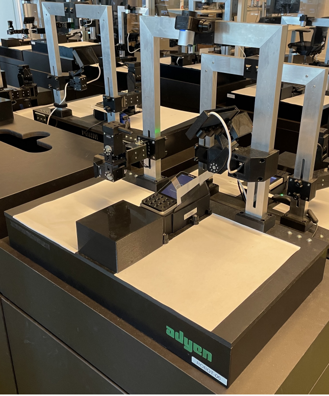
Fig. 5: Robot test setup at Adyen for the end-to-end testing of terminals by simulating real-life user interaction. The robot has the ability to insert, swipe or tap cards and provide input on the numeric pad and screen.
