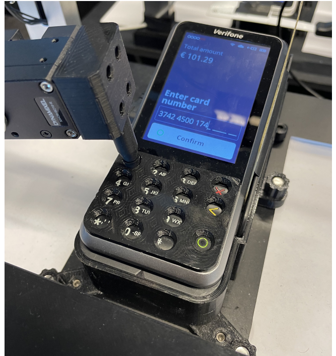
Fig. 7: Close-up view of the robot interacting with the terminal during a test.
