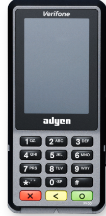
Fig. 4: Verifone P400Plus terminal, provided by Adyen to merchants for in-store payments. This specific model is used for the evaluation of GitFL.
