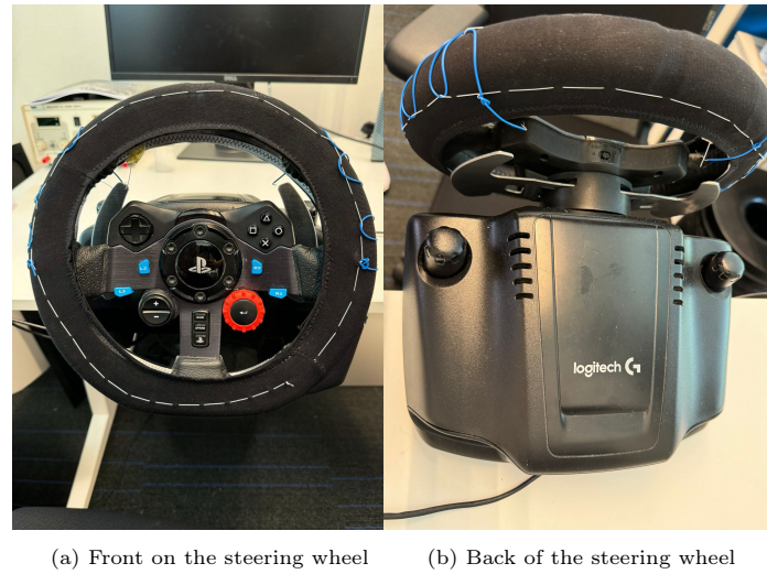
Figure 4.6: Illustration of how the wires are attached to the steering wheel to measure grip strength signals
