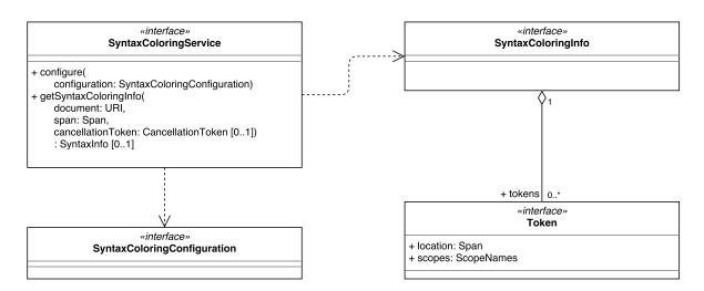
Figure 5.11: Overview of the AESI API for syntax coloring.
