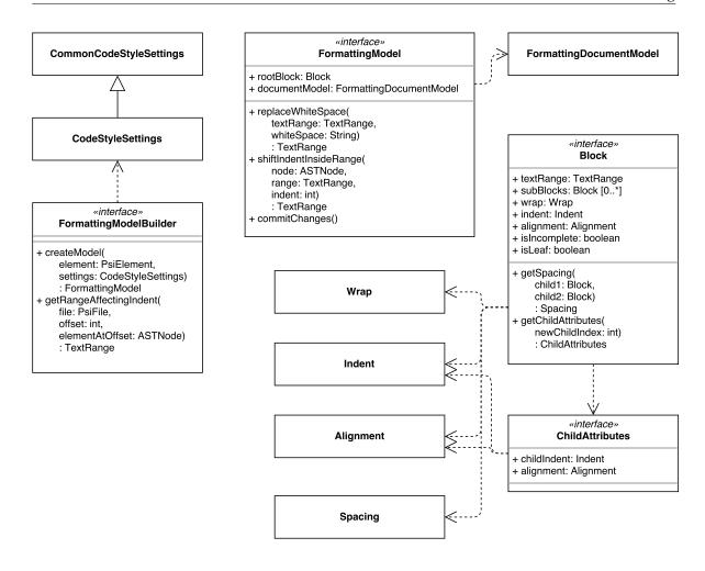
Figure A.23: Overview of the API for automatic formatting in IntelliJ.
