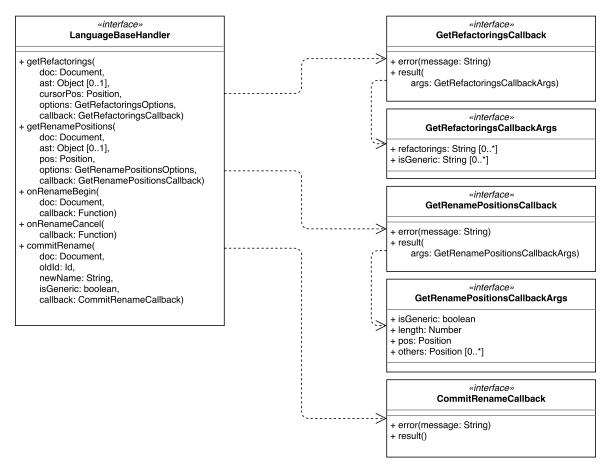
Figure A.32: Overview of the API for rename refactoring in Cloud9.
