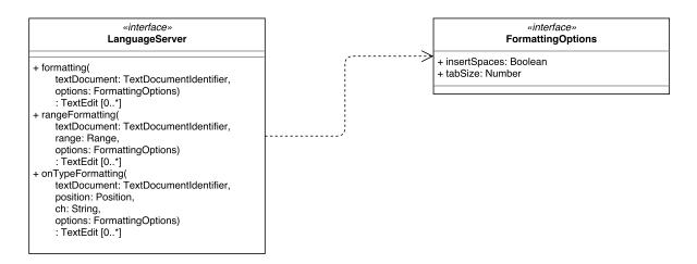
Figure A.26: Overview of the API for automatic formatting in LSP.
