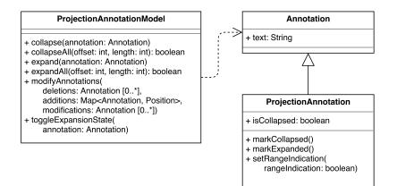
Figure A.4: Overview of the API for code folding in Eclipse.
