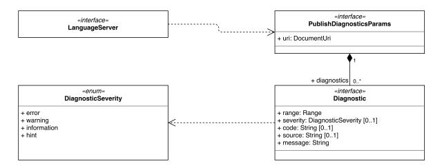
Figure A.40: Overview of the API for diagnostic messages in LSP.
