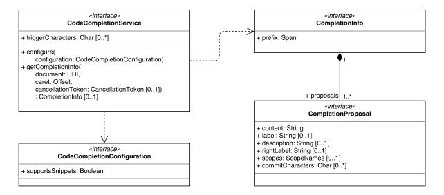
Figure 5.13: Overview of the AESI API for code completion.
