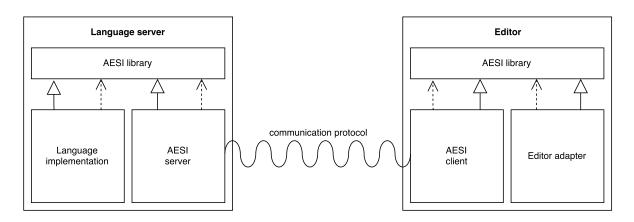
Figure 5.4: Custom communication between editor and language. An AESI server and client take the places of the editor adapter and language implementation respectively, and relay the requests and responses to one another.
