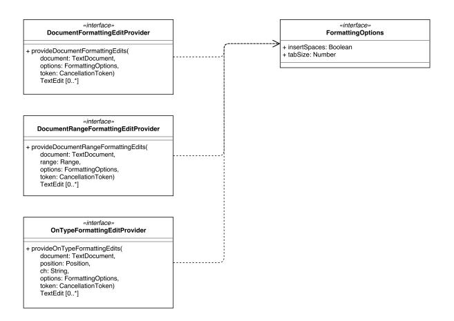
Figure A.24: Overview of the API for automatic formatting in VS Code.
