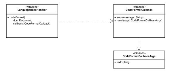
Figure A.25: Overview of the API for automatic formatting in Cloud9.
