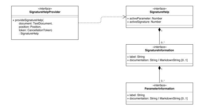
Figure A.19: Overview of the API for signature help in VS Code.
