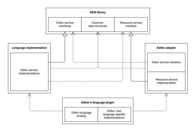
Figure 5.1: Diagram of the dependencies between a language and editor with AESI. The adapter calls the AESI editor service interfaces which are part of the language implementation, and the language implementation calls the AESI resource service which is implemented by the editor adapter. The editor's language plugin binds the language implementation and editor adapter together, and integrates them into the editor.
