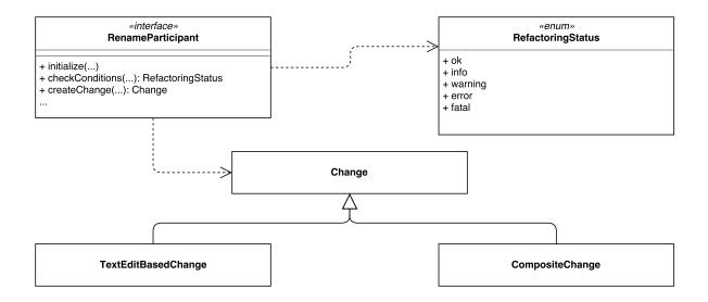
Figure A.29: Overview of the API for rename refactoring in Eclipse.
