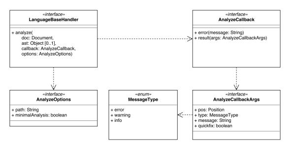
Figure A.39: Overview of the API for diagnostic messages in Cloud9.
