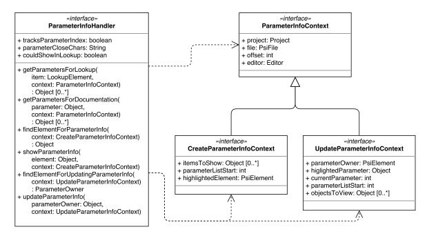
Figure A.18: Overview of the API for signature help in IntelliJ.
