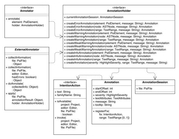
Figure A.38: Overview of the API for annotations in IntelliJ.
