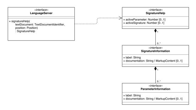
Figure A.20: Overview of the API for signature help in LSP.
