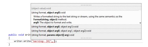
Figure A.16: Signature help in Visual Studio, highlighting the second parameter of the function.
