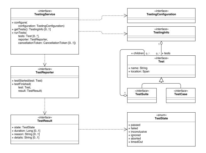
Figure B.7: Model for test discovery and execution.
