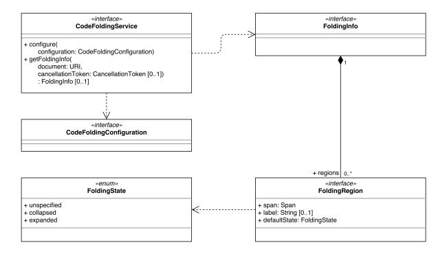
Figure B.1: Overview of the AESI API for code folding.
