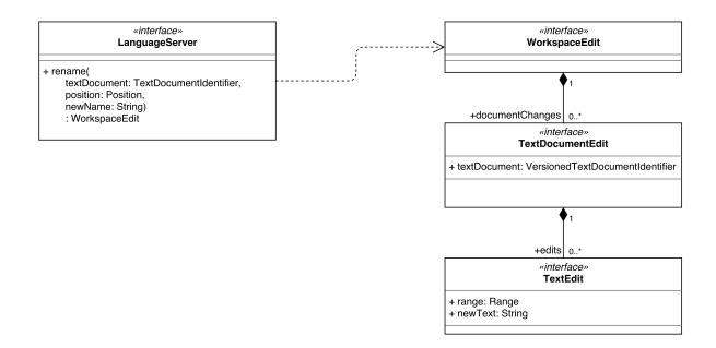
Figure A.33: Overview of the API for rename refactoring in LSP.
