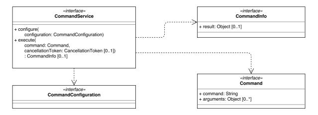
Figure 5.10: Model for the command service.
