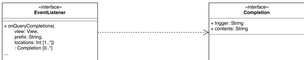
Figure 4.14: Overview of the API for code completion in Sublime.
