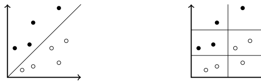
Figure 3.6: Data set with one multivariate split and three univariate splits showing the effectiveness of multivariate splits
