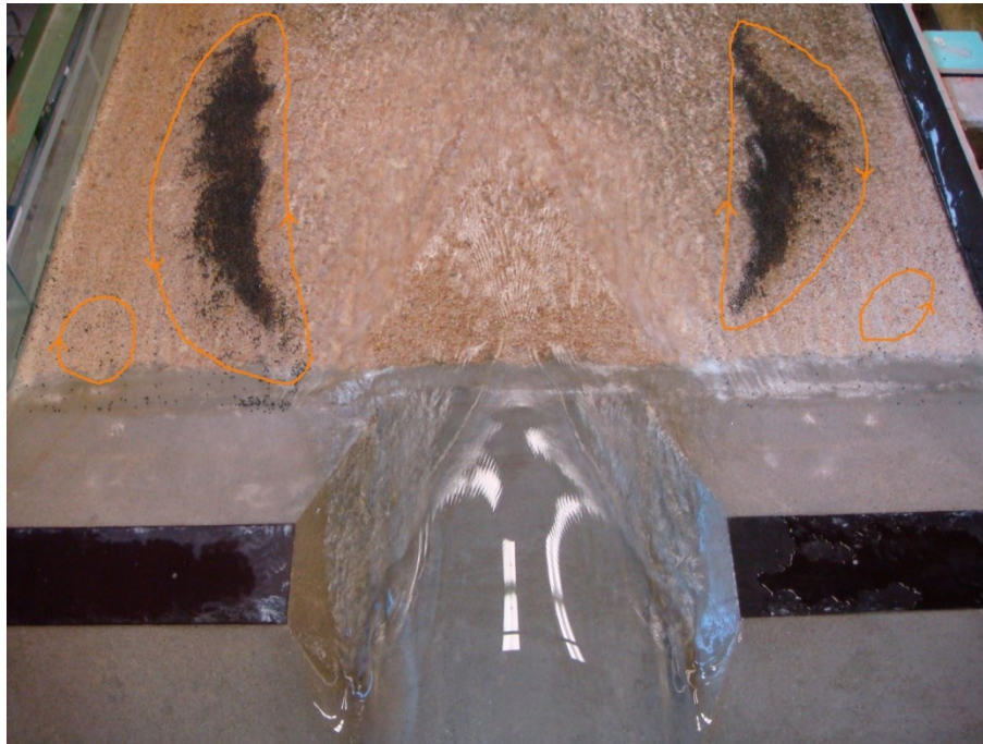
Figure 3.23 Breach flow pattern in weir flow condition ( Q = 20 l/s, case 5)
