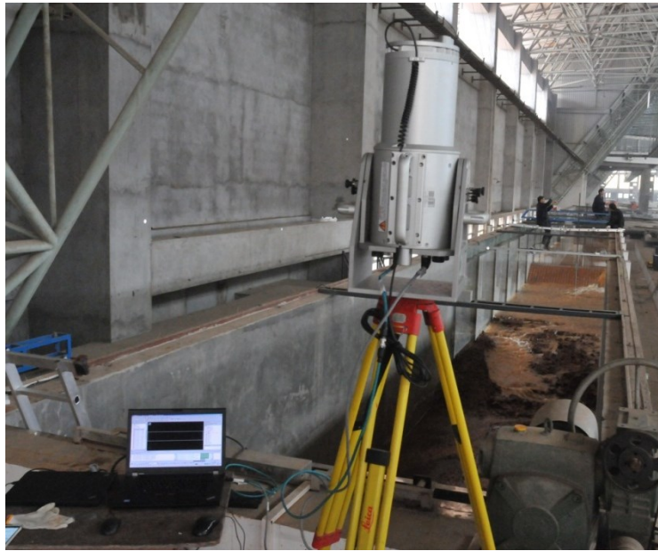
Figure 5.18 Three dimensional laser scanner systems
