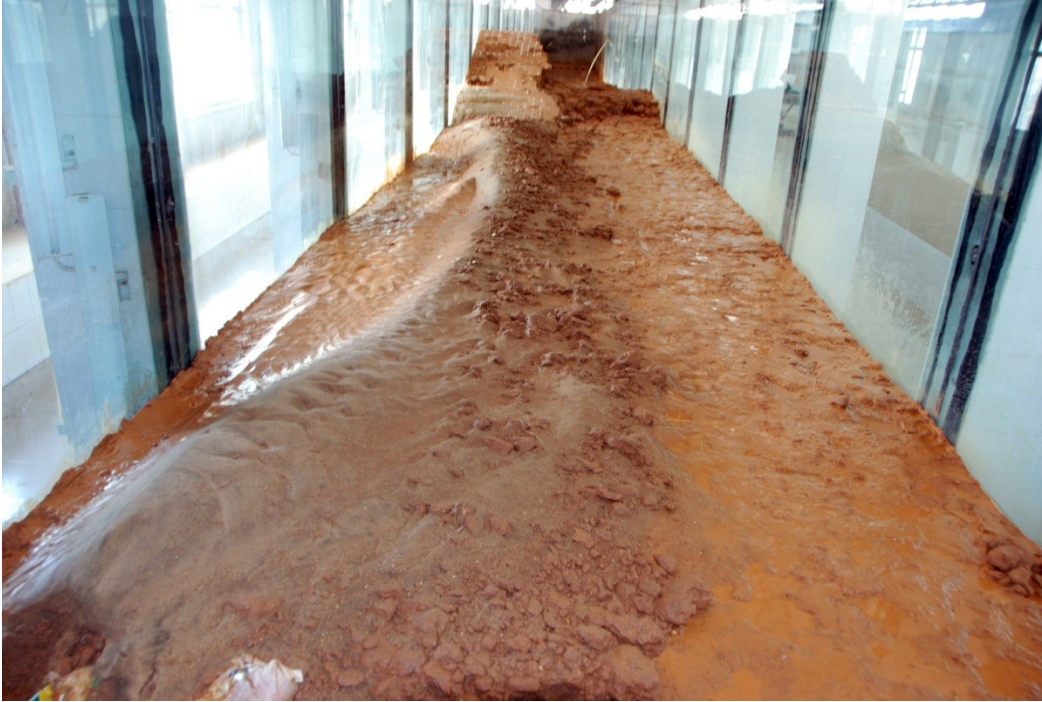
Figure 5.33 Final topography of Model 4 from the downstream overview
