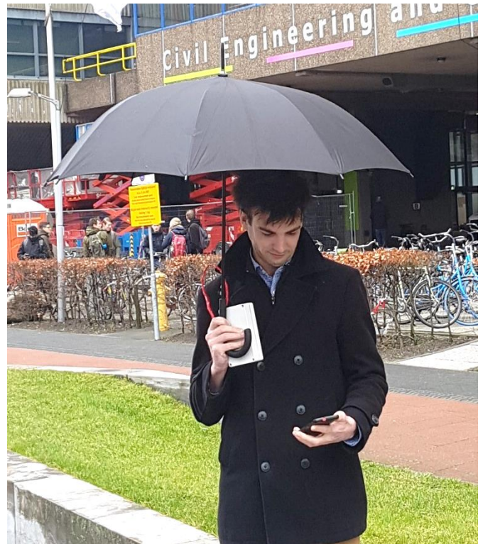
Figure 1: The author testing the umbrella in an urban area. The data measured are send to an application on the mobile phone.
