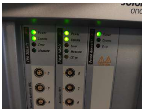
Figure 3.10: LEDs indicating a correct standby status of the Modulab XM after booting up. The second row, with labels "Comms" should be blinking.
