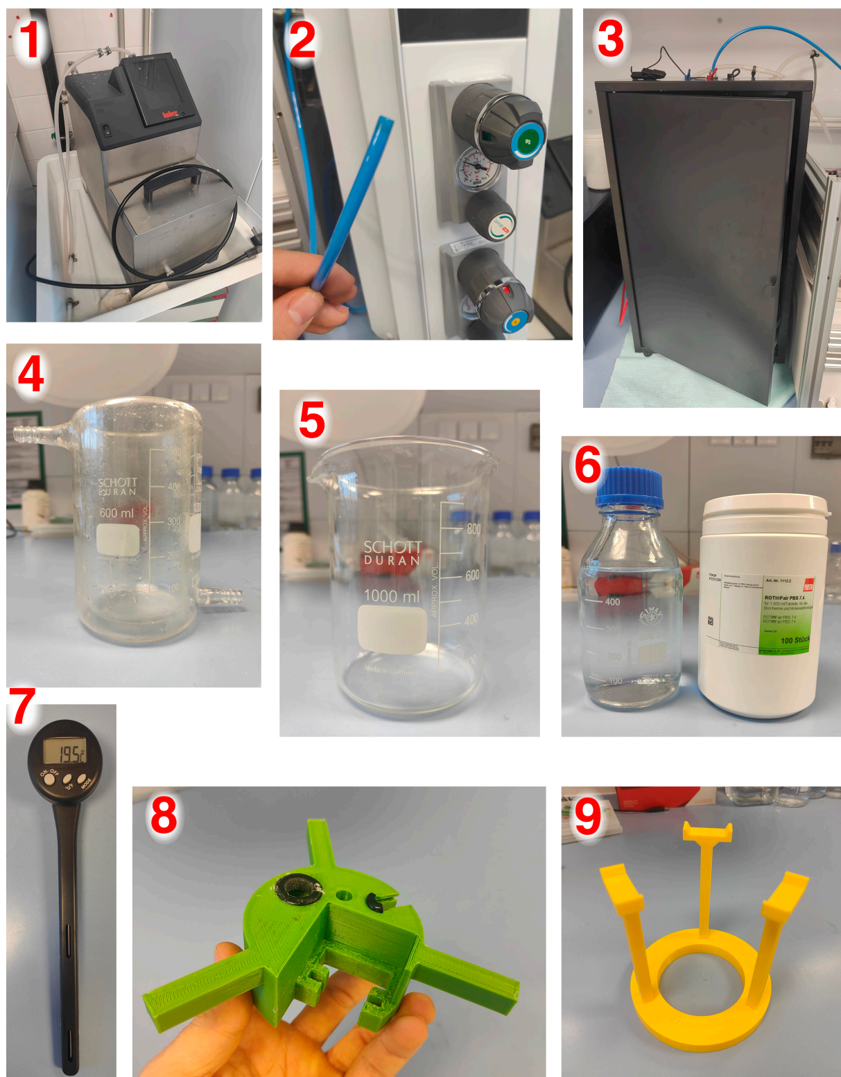
Figure C.2: Equipment items needed for all types of Electrode Characterization Testing 1. In numerical order: 1 - Thermostat, 2 - N 2 Gas Probe, 3 - Faraday Cage, 4 - Double Glass Walled Beaker, 5 - 1L Glass Beaker, 6 - PBS Solution, 7 - Thermometer, 8 - 3-Electrode Holder, 9 - 3-Electrode Holder Support
