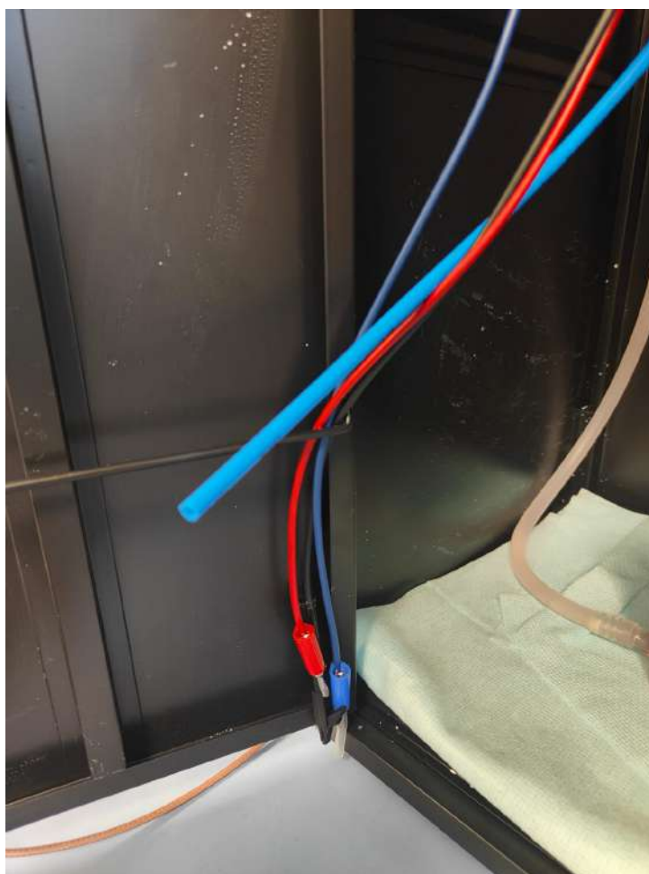
Figure 7.2: Use the thin beam on metal door of the faraday cage to hold and store all of the internal cabling. The N2 probe can also be held out of the way for easier operation with the cables' support, shown in the picture.
