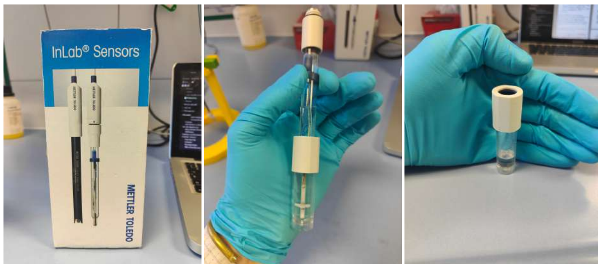
Figure 3.5: Glassy Carbon Ag/AgCl RE 's box from Metler Toledo. Remove the protective cap, and make sure to keep it upright to avoid spilling the storage solution.
