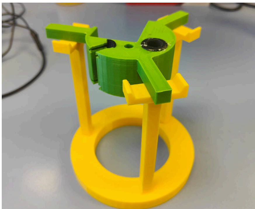
Figure C.15: Pictures of the 3-Electrode Holder assembled with the corresponding rubber rings to softly grip the electrodes without damaging them.
