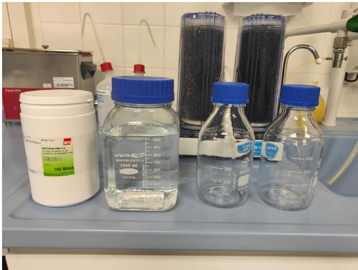
Figure 7.7: Equipment needed to make and store fresh PBS according to the protocol. It is best to make fresh PBS when two of the 0.5L jars are empty, as each tablet is meant for 1L of DI water.
