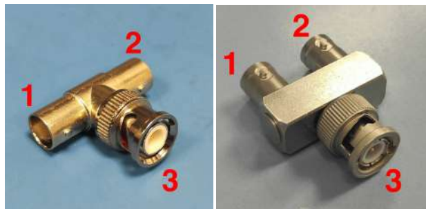
Figure 4.7: Left: T-splitter - AVOID if possible. Right: Y-splitter - BETTER option
