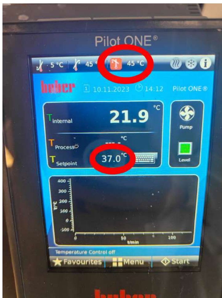
Figure 2.7: Check the safety temperature limit (top row) and the Setpoint T (in yellow, in the centre square). This is how the thermostat screen should look before starting the flow of heating liquid.
