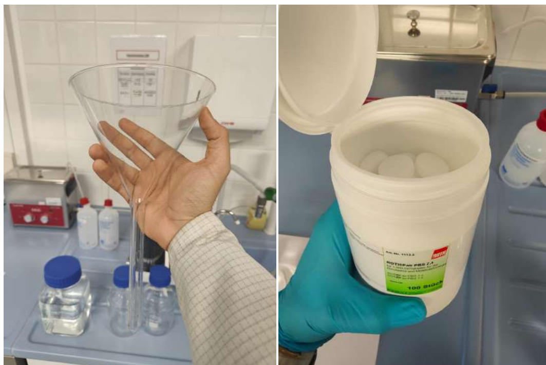
Figure 7.8: (Left) Large glass funnel, optional (but useful) for safely transferring PBS between jars. (Right) CarlRoth ROTI PBS pH 7.4 tablets are meant for 1L of DI water.
