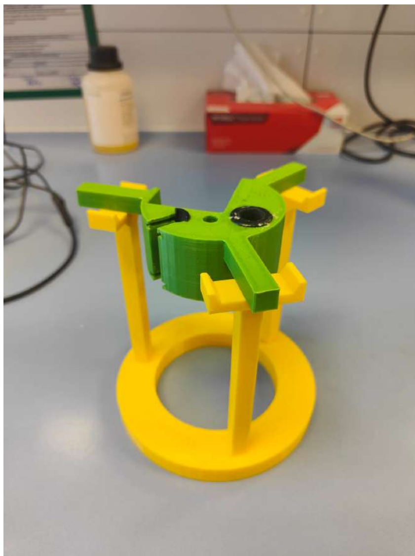
Figure 2.11: Place the electrode holder (green) on the workbench with the help of the support (yellow)
