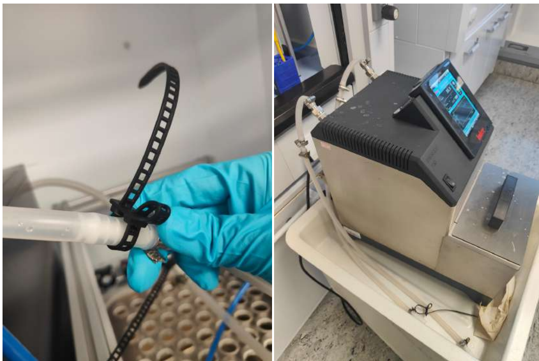
Figure 7.6: Loosen the plastic fasteners and disconnect the tubing sections. The tubes connected directly to the thermostat may be kept within the tray, to keep minor spills from falling on the floor
