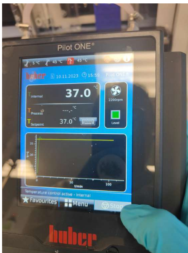
Figure 7.1: Turn off the thermostat's pump to stop the heating liquid from circulating the tubing. Press the stop button (bottom right corner) and then the Ok button that will show on the screen
