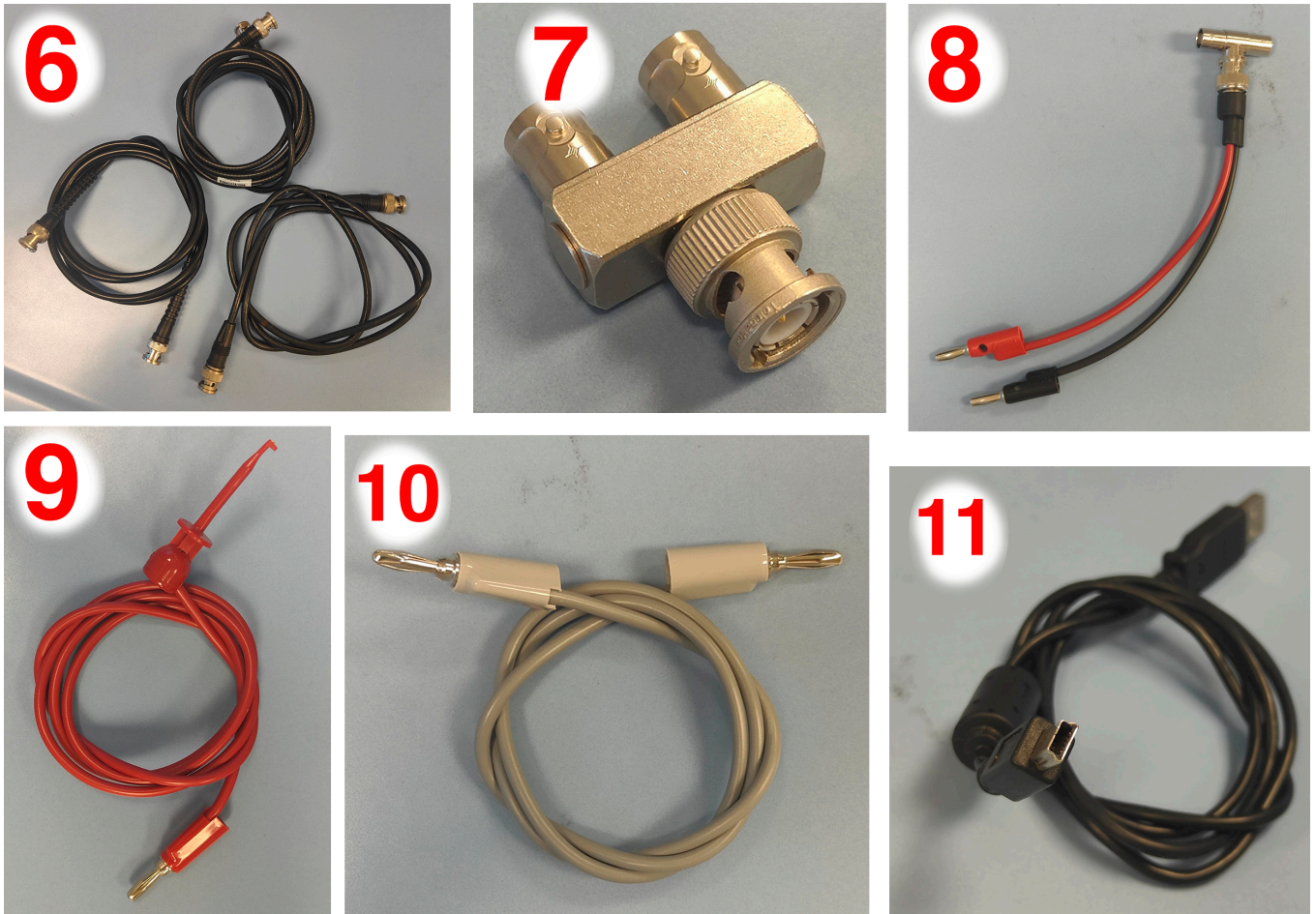
Figure C.7: Equipment for VT Testing 2. In numerical order: 6 - 3 BNC cables, 7 - 1 BNC cable signal Y-splitter, 8 - 1 BNC to Banana +,- adapter, 9 - 1 Banana to Hook cable, 10 - 1 Banana to Banana cable, 11 - 1 MINI USB to USB cable
