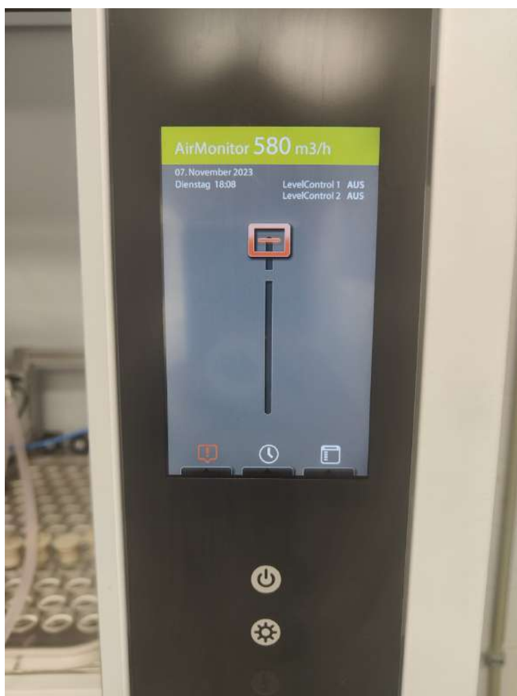
Figure 2.3: Panel showing the window pane is open, as the bar is at the top
