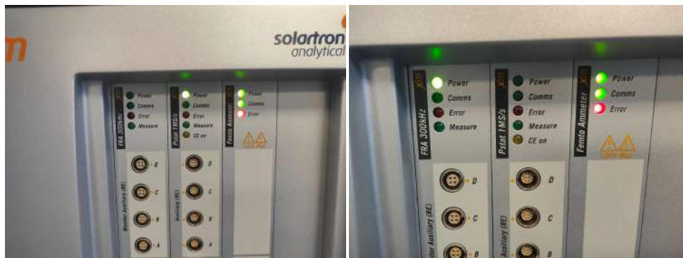
Figure 3.11: Different status of the Modulab XM, while which it should not be operated. They may show during boot up, or after booting up if this step was unsuccessful, or if the system freezes/bugs out during an experiment.
