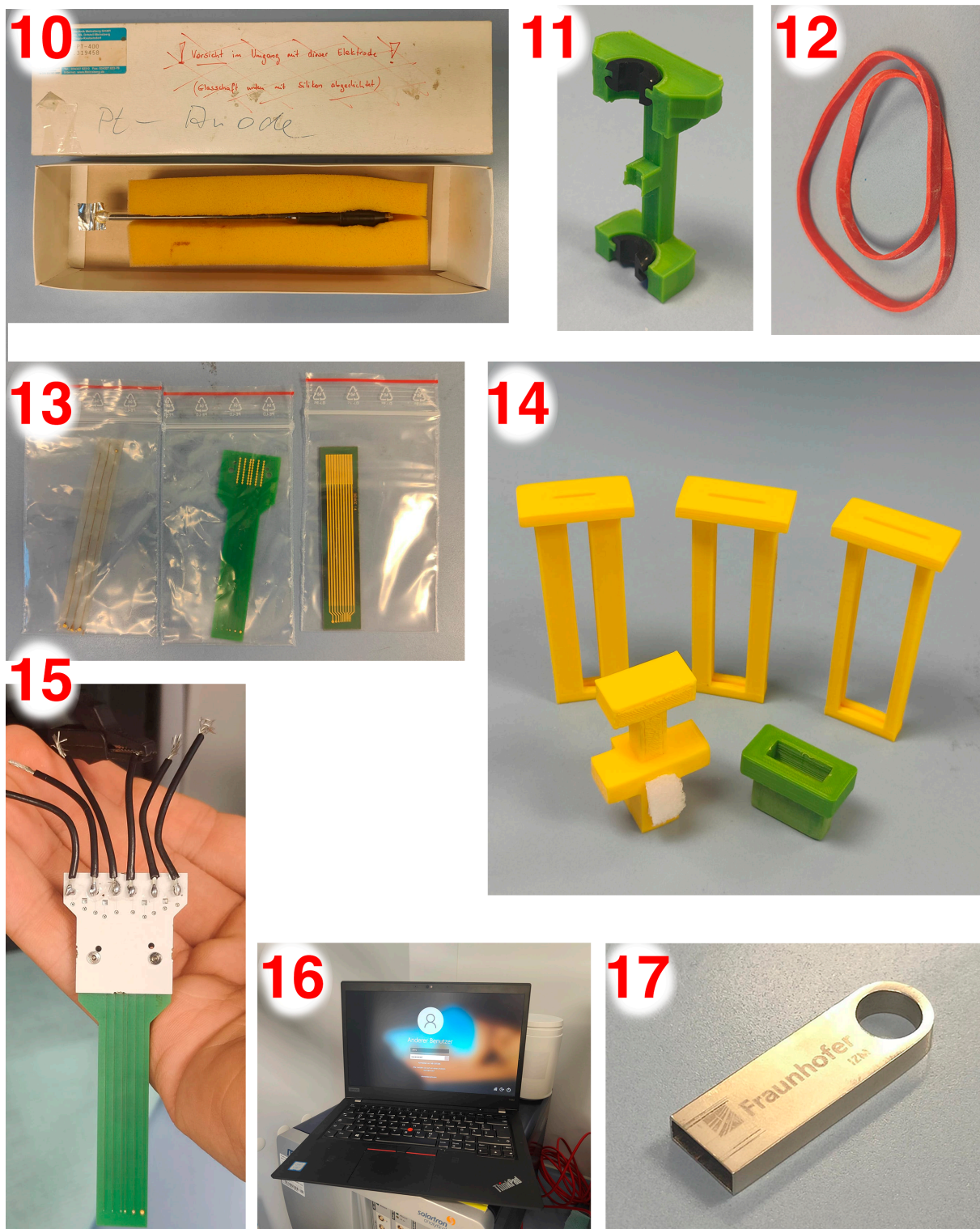
Figure C.3: Equipment needed for all types of Electrode Characterization Testing 2. In numerical order: 10 - Pt flag foil large return electrode (CE), 11 - CE Lock, 12 - Rubber Band, 13 - WE Samples, 14 - WE Sample Holder, 15 - WE Connector, 16 - Working Laptop NB-SIIT086, 17 - USB Thumbstick Drive
