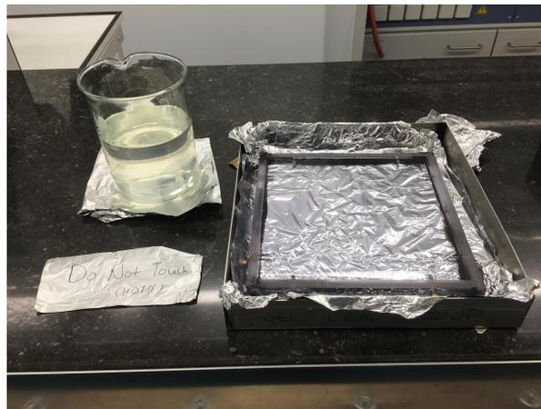
**Figure 3.4:** Coating casting process showing the solidified coating in a beaker and the melted coating in a polycarbonate plate mould inside the metal tray
