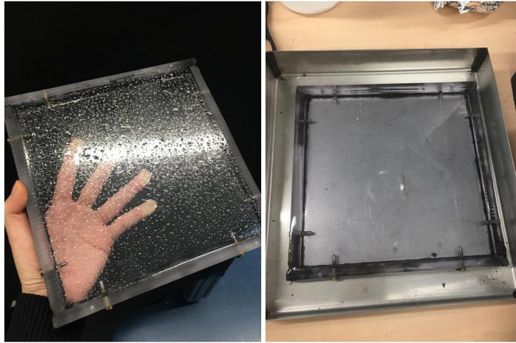
Figure 3.5: Damaged coating surface before and after remelting
