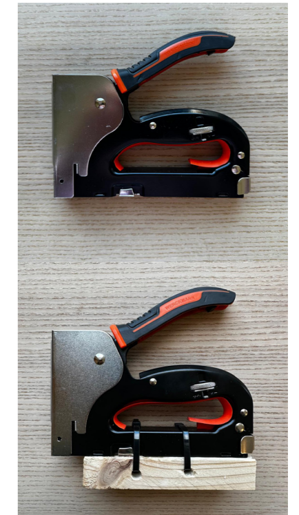
Figure 30: Adapted staple gun to make stapling stabler and safer. (top: old configuration, bottom: new configuration).
