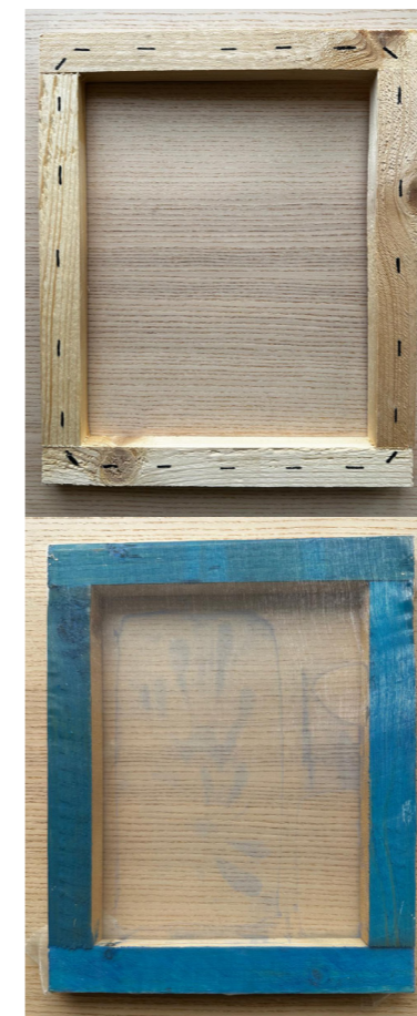
Figure 29: New flat wooden frame design with embedded instructions (a blue side and staple markings).
