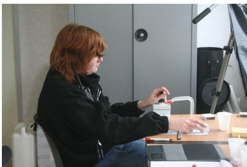
Picture 8.6. Operating the wave overtopping simulator by means of a joystick and list of times when to open the valve.
