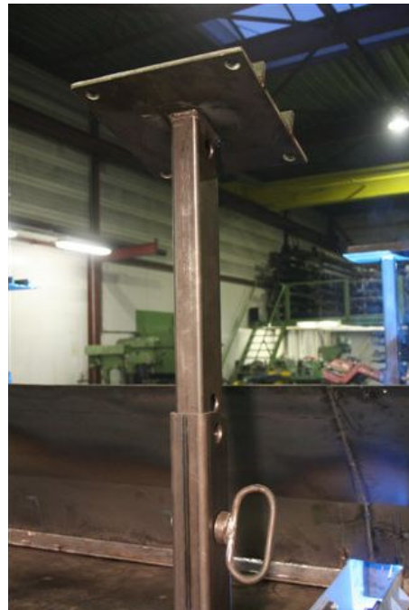
Picture 7.6. Adjustable leg rear side (upside down). Plate was later made rotational.
