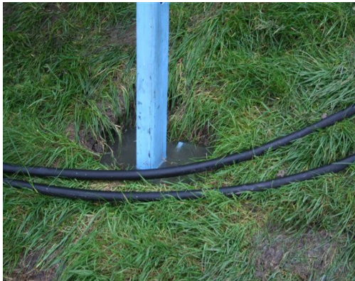
Picture 7.16. Subsidence of the legs into the clay after being loaded a few times with 14 m 3 of water.
