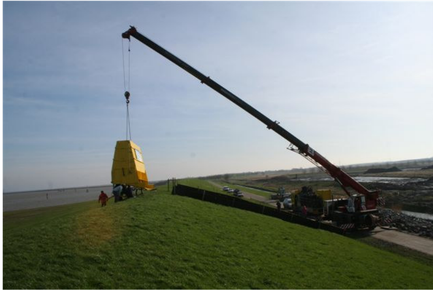
Picture 8.3. Placing the simulator on the test section by a large crane.
