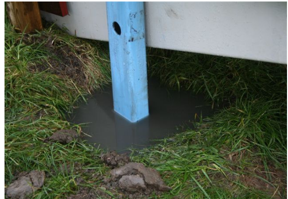
Picture 7.16. Subsidence of the legs into the clay after being loaded a few times with 14 m 3 of water.
