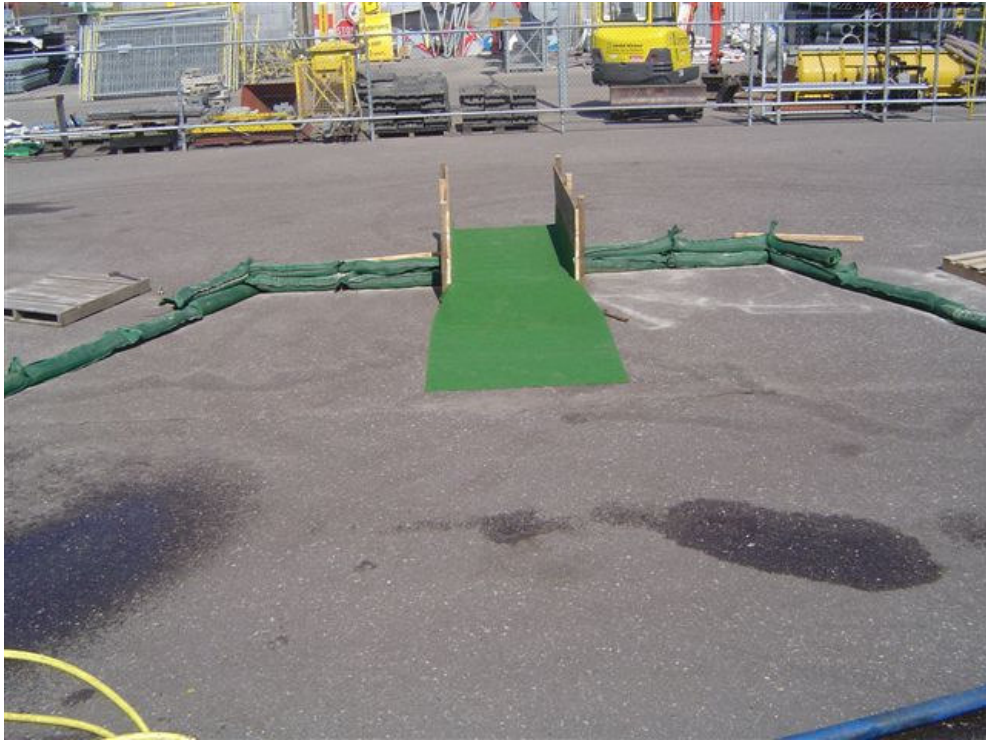
Picture 4.5. Set-up of calibration flume, surrounded by sand bags
