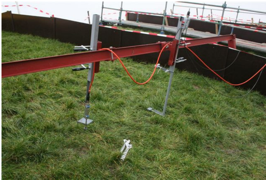
Picture 9.1. Steel beam over test section with instruments mounted to it.
