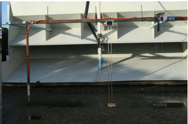
Picture 7.12. From right to left in front of the simulator: electromagnetic velocity meter EMS, conventional wave gauge and new wire flow depth meter.
