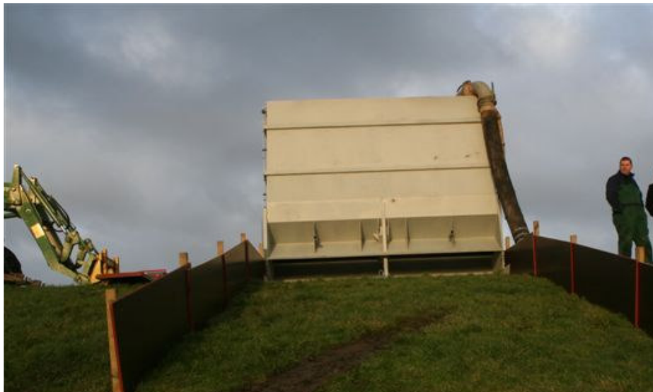
Picture 7.14. Wave overtopping simulator installed on dike and ready for action on the calibration day.
