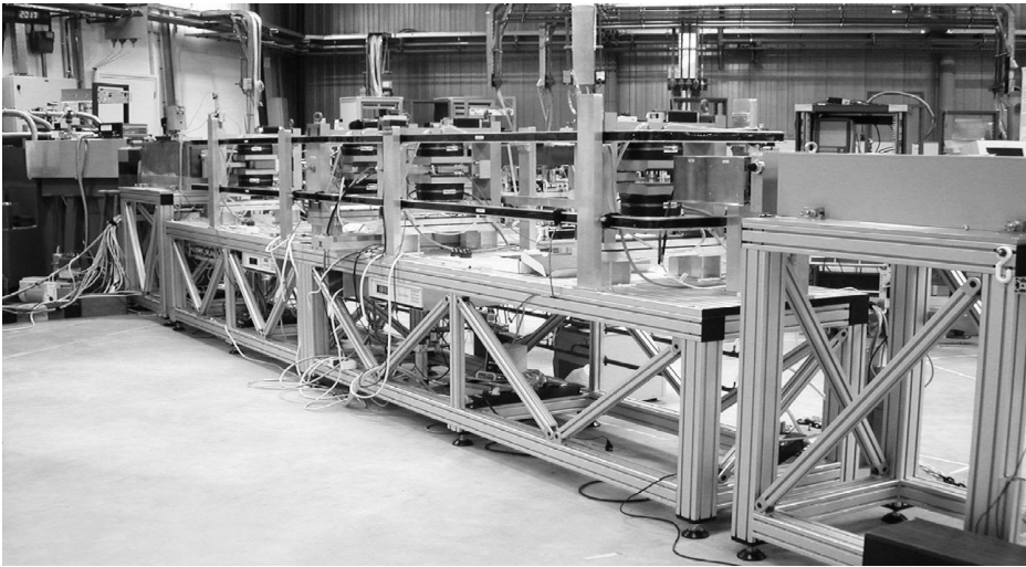
Figure 5.1: Photo of the SESANS setup at the Reactor Institute Delft, with the neutron guide exiting the reactor hall at the left. A crystal monochromator uses the Bragg condition to select a wavelength at a specific angle, after which a polarizer selects neutrons that have the same combination of their spin-eigenstates. Two magnets comprise the first magnetic region encoding the neutron spin, which can be described classically as Larmor precession or quantum-mechanically as the vertical separation of two neutron eigenstates. The selected magnetic field strength is proportional to the desired spin-echo length. A sample is placed on a translation table and moved in and out of the beam, in order to measure both empty beam and sample under equal conditions. Two magnets to the right form the second magnetic region decoding the neutron spin. This region has a geometry identical to the first, but with opposite field values. The echo condition is achieved by fine-tuning the four magnets with respect to each other. The polarization is measured by a combination of analyzer and detector.
