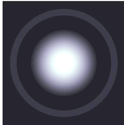
Figure 1.1: Computer generated image of the Airy diffraction pattern, which is observed when waves exit a circular aperture with a diameter in the order of the wavelength. The intensities of the pattern are by determined by a Fourier transform of the shape of the aperture, which yields a damped first order Bessel function. The bright central region, called the Airy disk, is surrounded by weak concentric rings of decreasing intensity.
