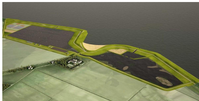
Figure 4.14: Concept photo of double dike at Eems-Dollard [3].
