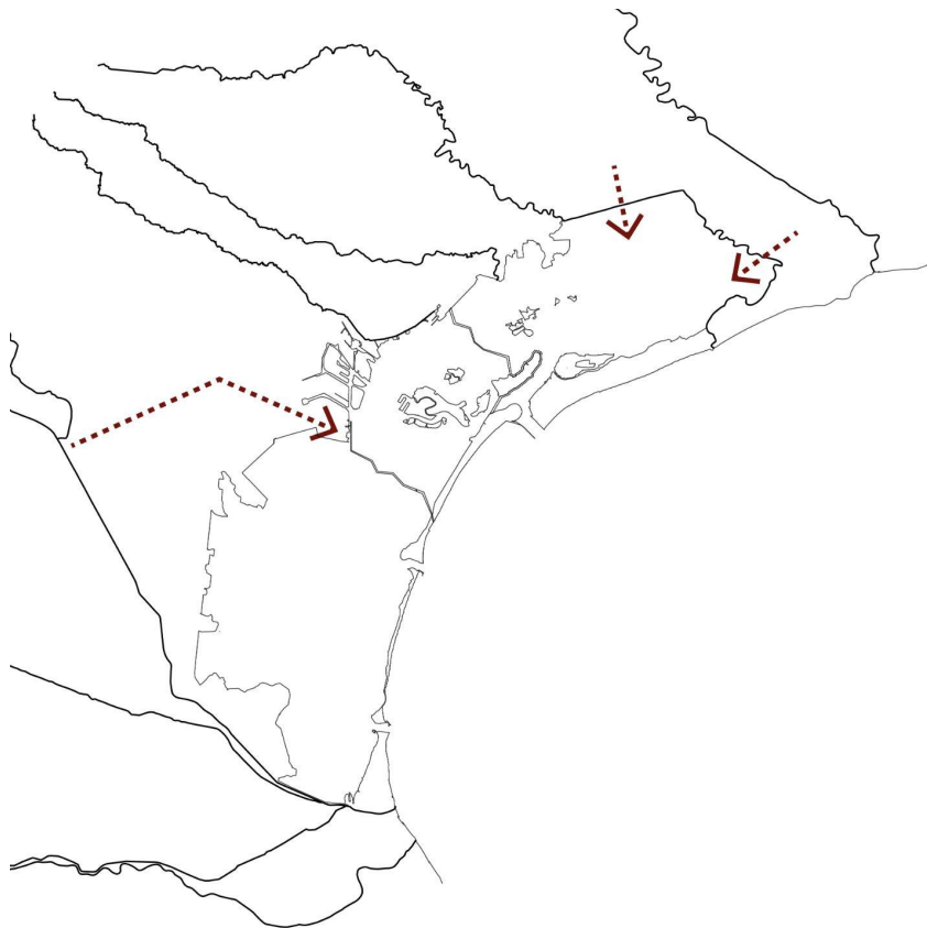
Figure 4.9: Implementation of the new meandering Brenta river and the possible debouching location of the Piave river. The Brenta will flow into the lagoon just below the southern wide green dike where it will develop its own delta. The Piave river can be combined with the Sile river or flow into the northern part of the lagoon.
