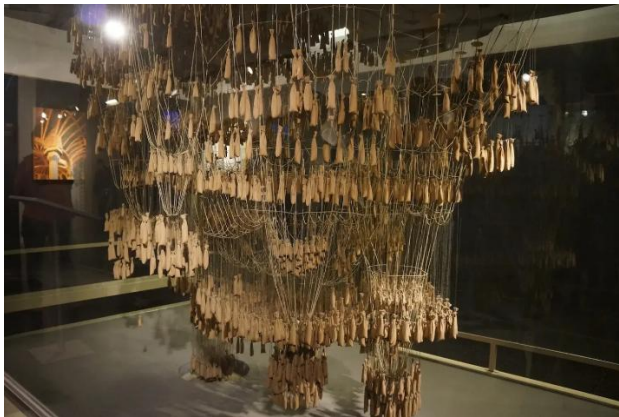
Figure 8: Antoni Gaudí - Hanging Chain Model for La Sagrada Família, Barcelona, Spain. (Source: Zexin & Mei, 2017).
