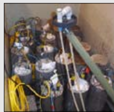
Test pieces used by Koleva in the climate basin at the faculty of Aerospace Engineering being sprayed with de-icing salts. Koleva investigated the effect of cathodic protection under such conditions.
