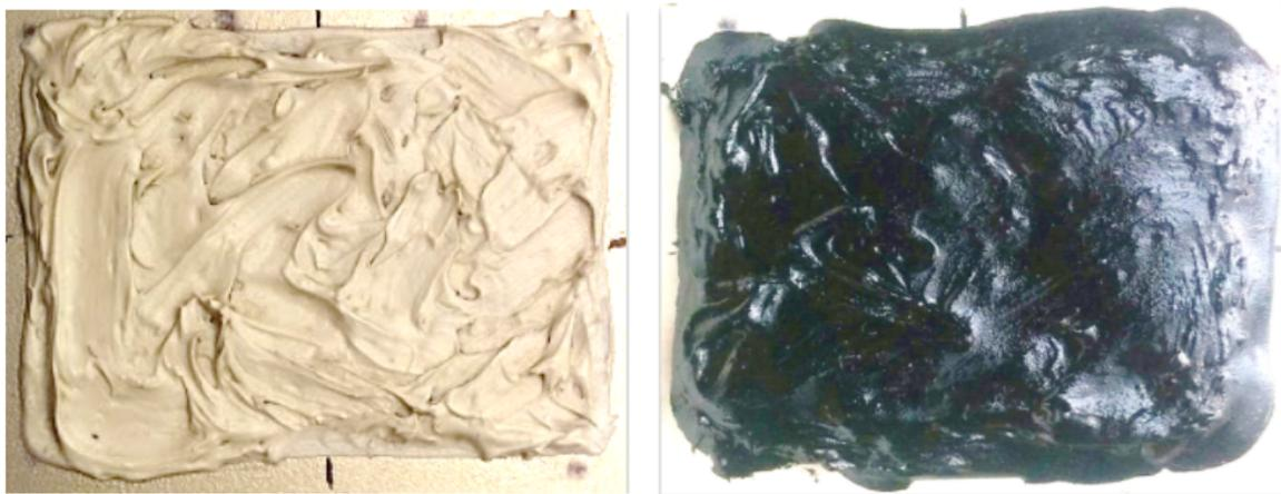
Figure 6.1: On the left, the layer of lead white paint on GLARE substrate. On the right, the finished sample with bone black applied over the lead white paint layer.
