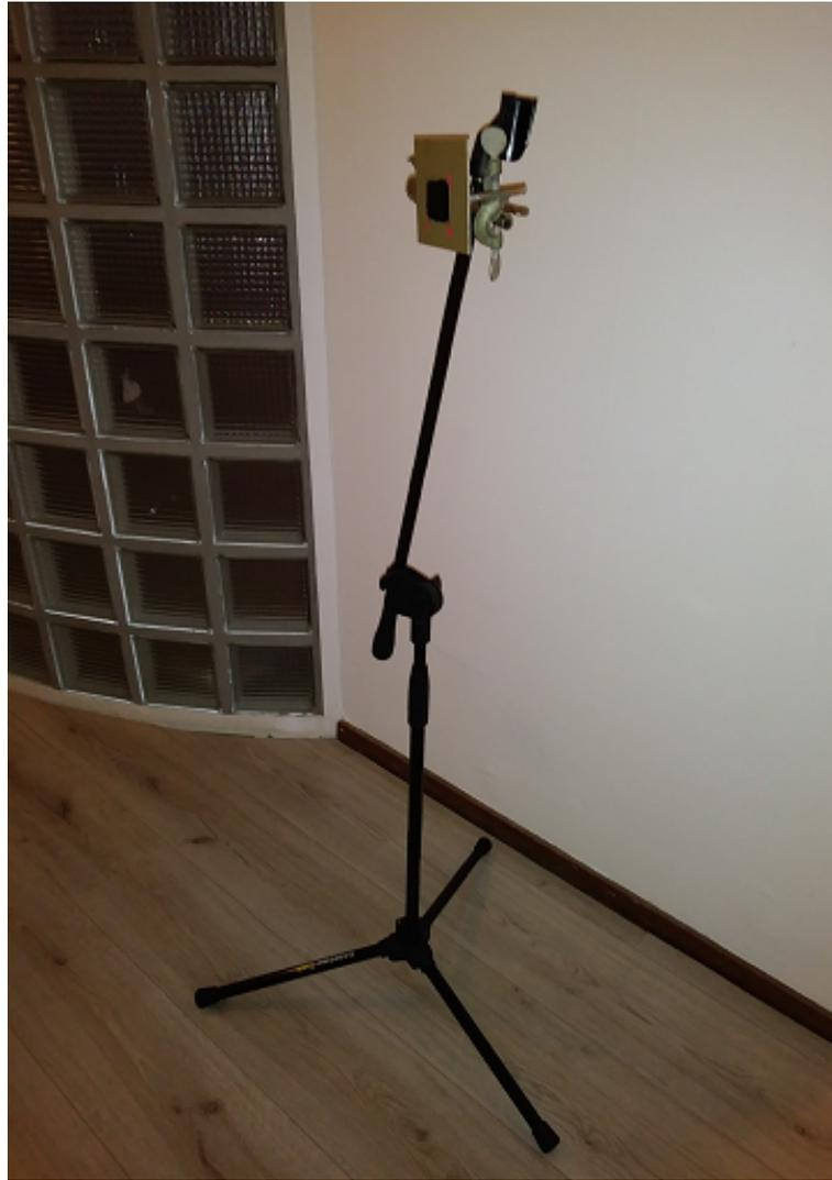
Figure 6.2: The sample mount was selected as a telescoping microscope stand with clamp holders for easy rotation of the sample on all axes.
