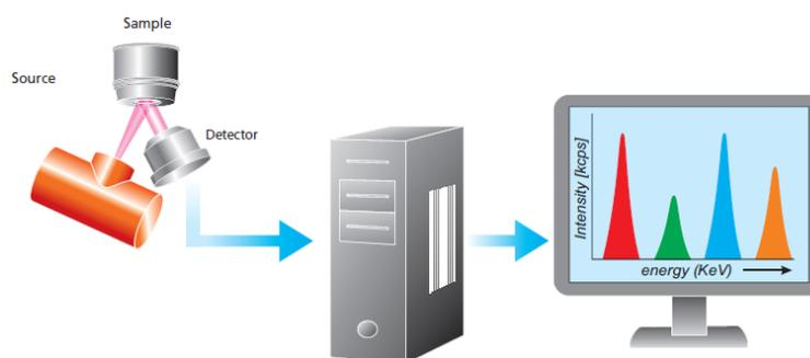
Figure 3.5: Schematic of a typical XRF setup
