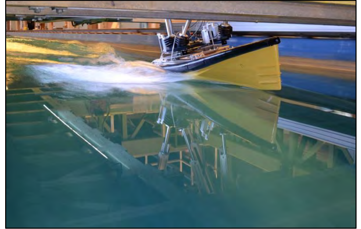
Figure 3 Model test run (Stage 1, Fr = 1.05 , \phi = 12 deg)
