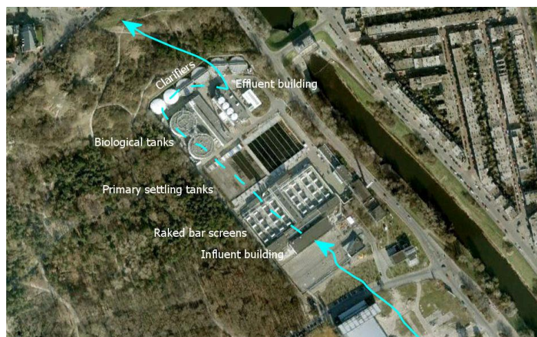
Figure 7.4: The treatment types of STP Houtrust.
