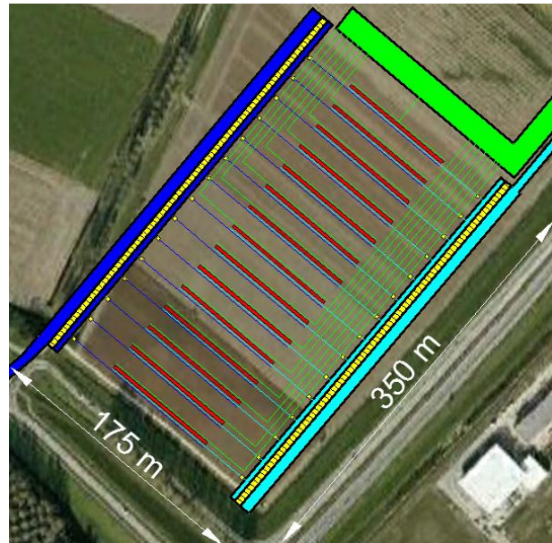
Figure 8.2: The 25 MW RED power plant configuration.
