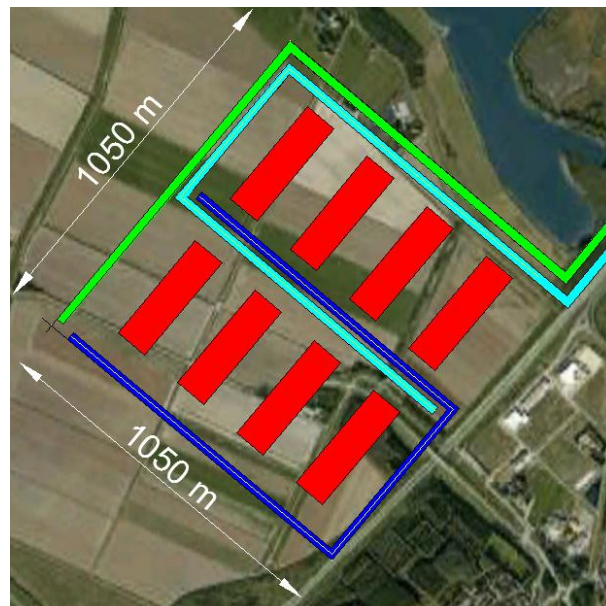
Figure 8.3: The 200 MW RED power plant configuration.
