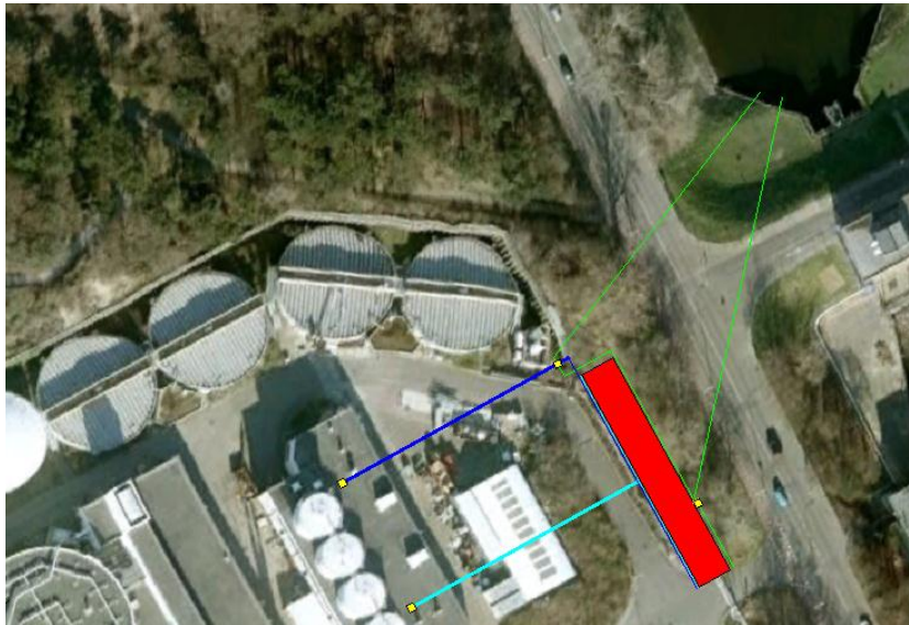
Figure 7.5: The position of the pumps, pipes, turbines and membrane stack of the 1 MW PRO power plant.
