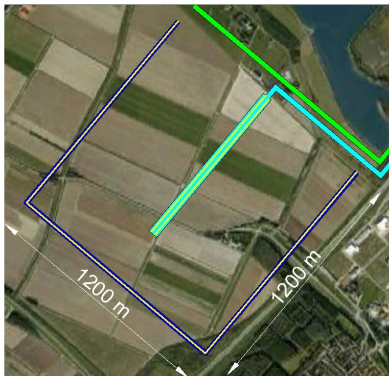
Figure 6.23: The position of the pre-treatment facility in the case of a 200 MW PRO power plant.
