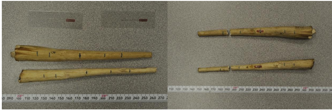
Figure 3-8 Tensile Test for Pneumatophore; picture at the top: Shimadzu test machine with root samples; on the left bottom: samples before test with strain gauge; on the right bottom: samples after test;
