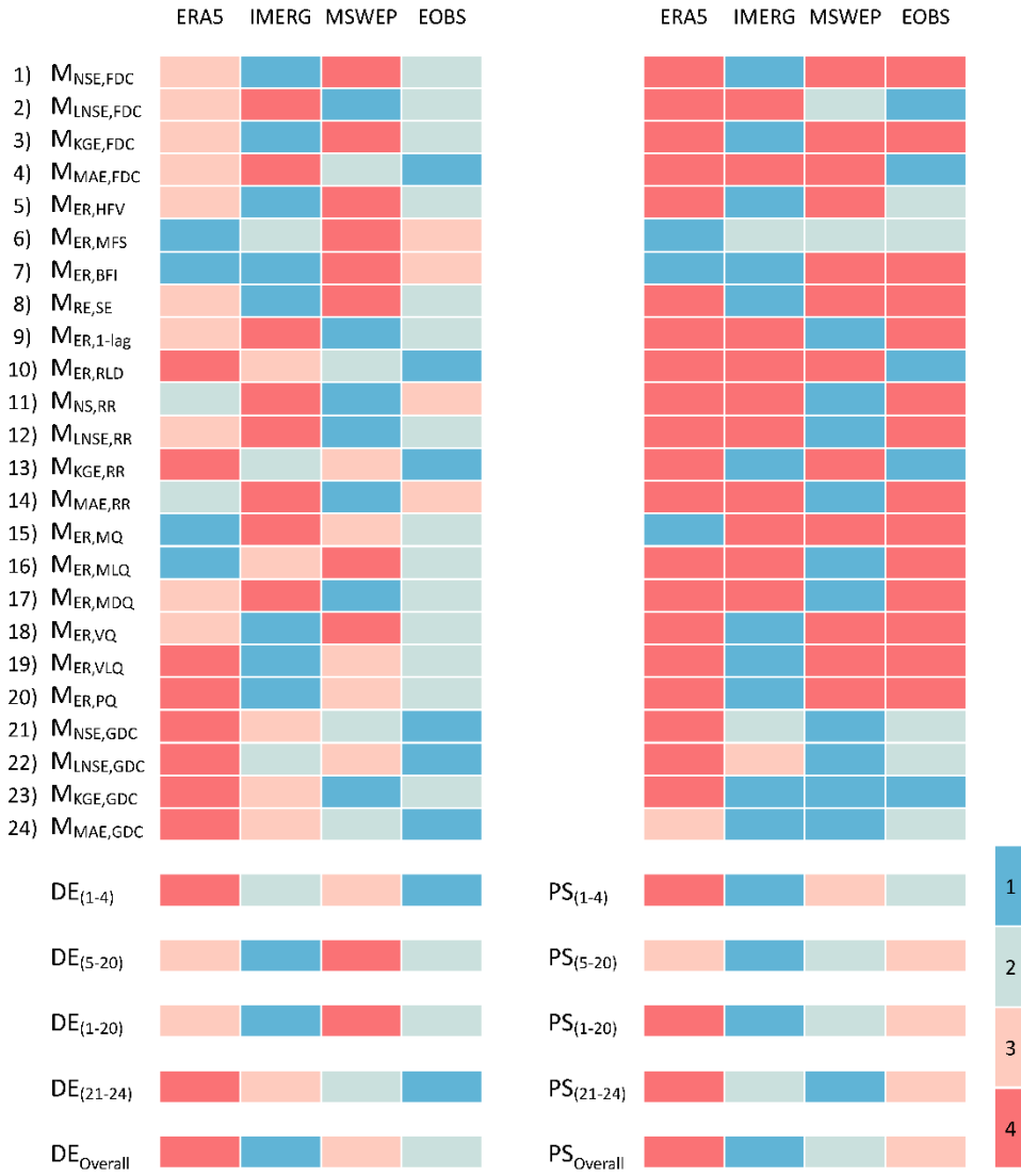
Figure 4.6. The performance of gridded precipitation products to reproduce discharge and groundwater signatures evaluated using signatures-based metrics (Table 4.2, row 3-17) represented individually and combined using criteria: (1) the Euclidean distance (DE) on the left side and (2) the Percentage score (PS) on the right side. Performance is ranked on a scale from 1 to 4, with 1 representing the most suitable product while 4 representing the least one
