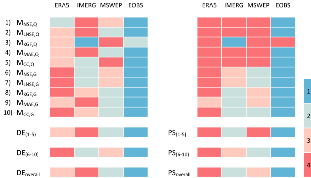
Figure 4.5. The performance of gridded precipitation products to reproduce discharge and groundwater levels evaluated using timeseries based metrics (Table 4.2, at 1 and 2) represented individually and combined using criteria: (1) DE on the left side and (2) PS on the right side. Performance is ranked on a scale from 1 to 4, with 1 representing the most suitable product while 4 representing the least one
