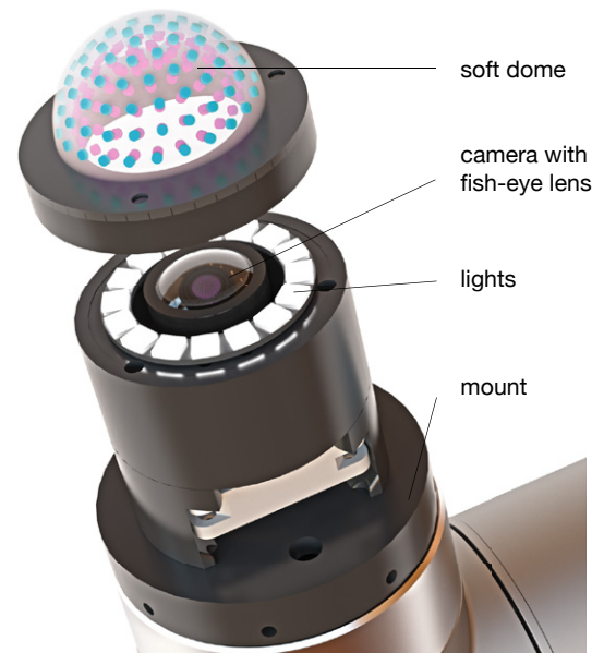
Fig. 5: Render of the fingertip assembly with the tactile sensing dome, fish-eye camera and LED lights, reprinted from [33].
