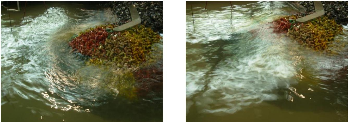
Figure 8.3 – Images of the roundhead with dolos during test RB-B2
