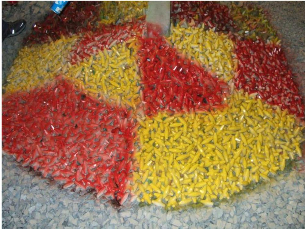
Figure 7.3 – Roundhead model of the covering alternative with 45-tonne Core-Loc
