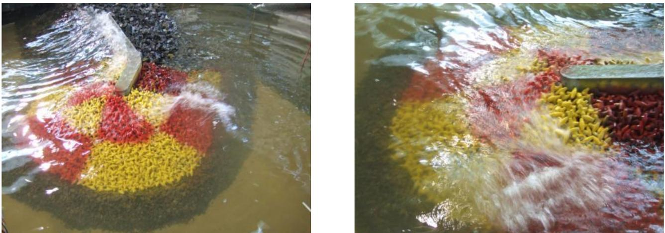
Figure 8.11 – Images of the roundhead with Core-loc during test RB-B2
