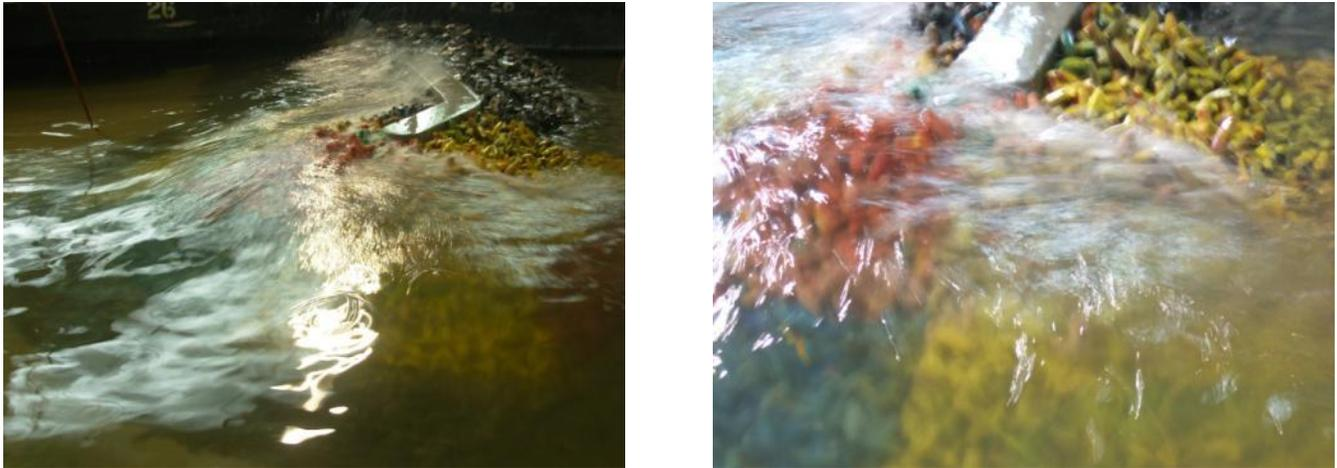
Figure 8.4 – Images of the roundhead with dolos during test RB-A2
