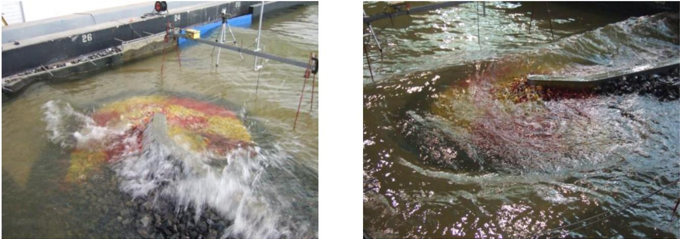
Figure 8.16 – Images of the roundhead with Core-loc during test RB-A4
