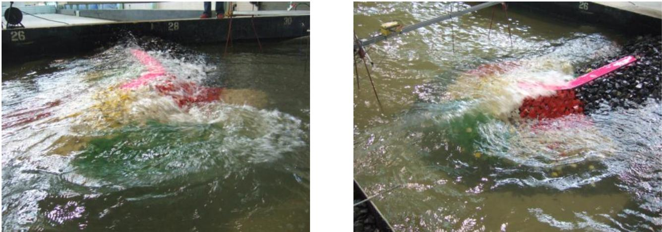
Figure 8.26 – Images of the roundhead with antifer cubes during test RB-A5
