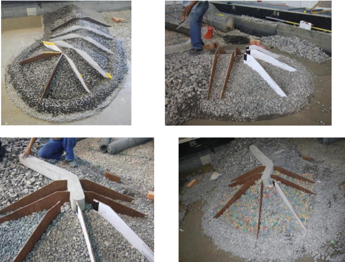
Figure 7.1 – Construction sequence of the roundhead model
