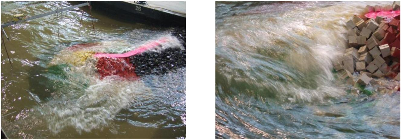
Figure 8.24 – Images of the roundhead with antifer cubes during test RB-B4
