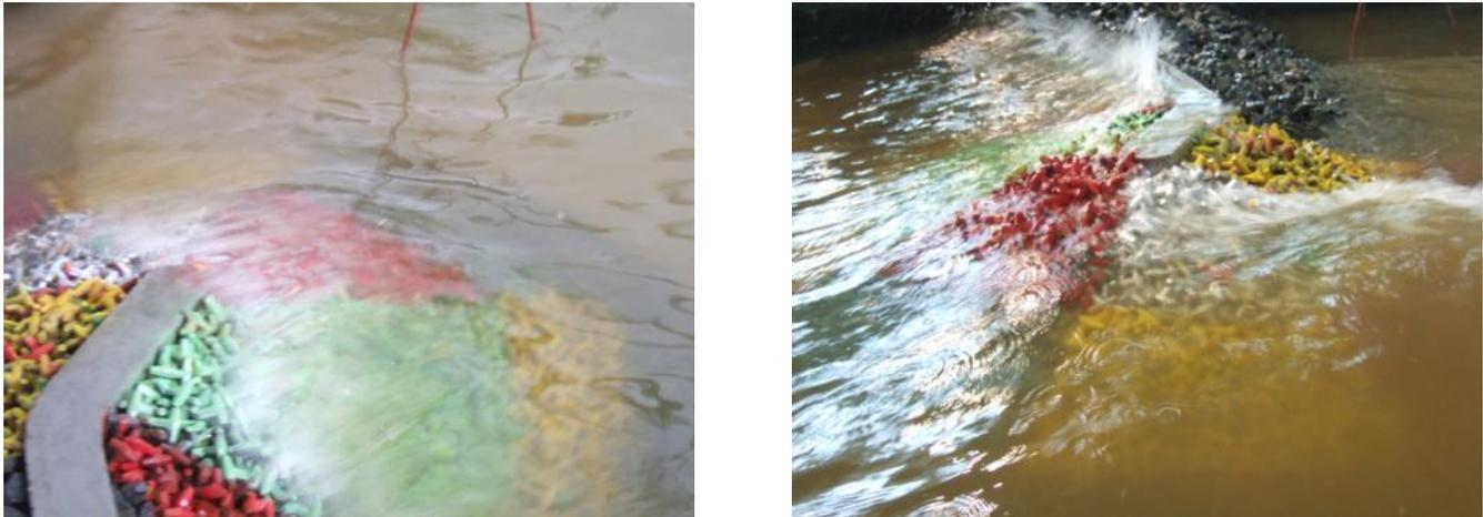
Figure 8.8 – Images of the roundhead with dolos during test RB-B4
