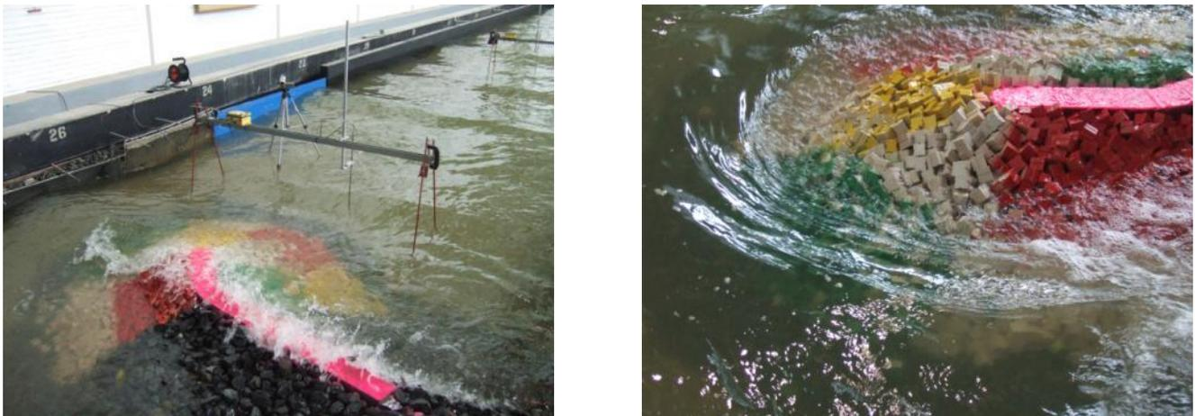
Figure 8.25 – Images of the roundhead with antifer cubes during test RB-A4
