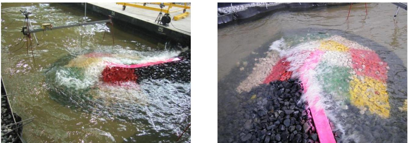
Figure 8.23 – Images of the roundhead with antifer cubes during test RB-A3
