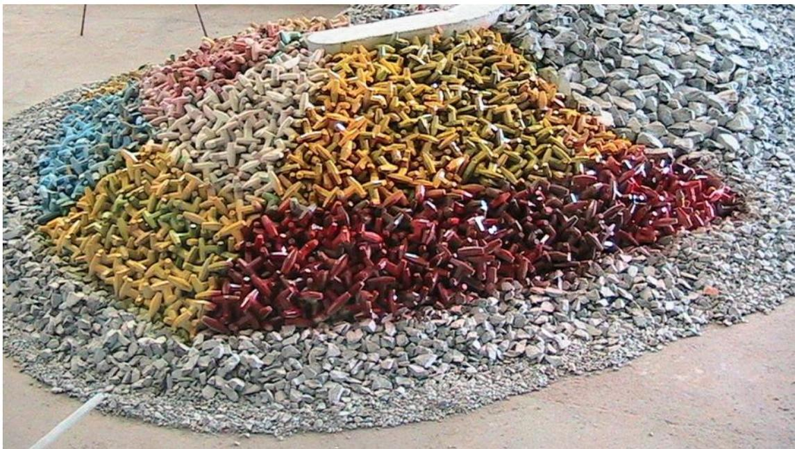
Figure 7.2 – Roundhead model of the covering alternative with 36-tonne dolosse
