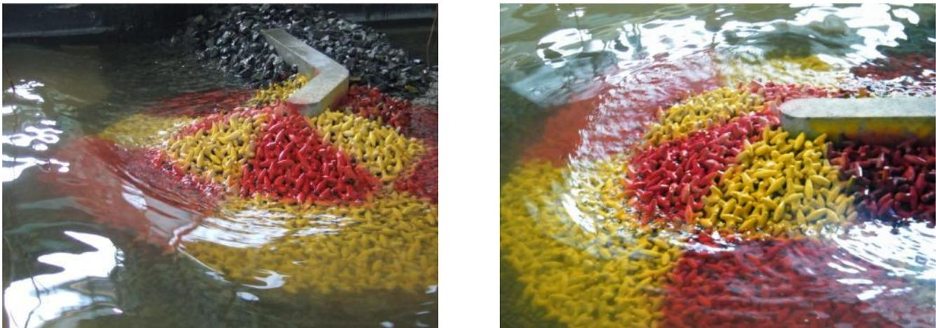
**Figure 8.9 – Images of the roundhead with Core-loc during test RB-B1**
