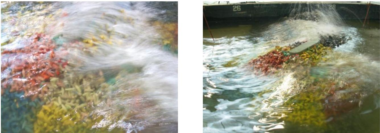
Figure 8.7 – Images of the roundhead with dolos during test RB-A4
