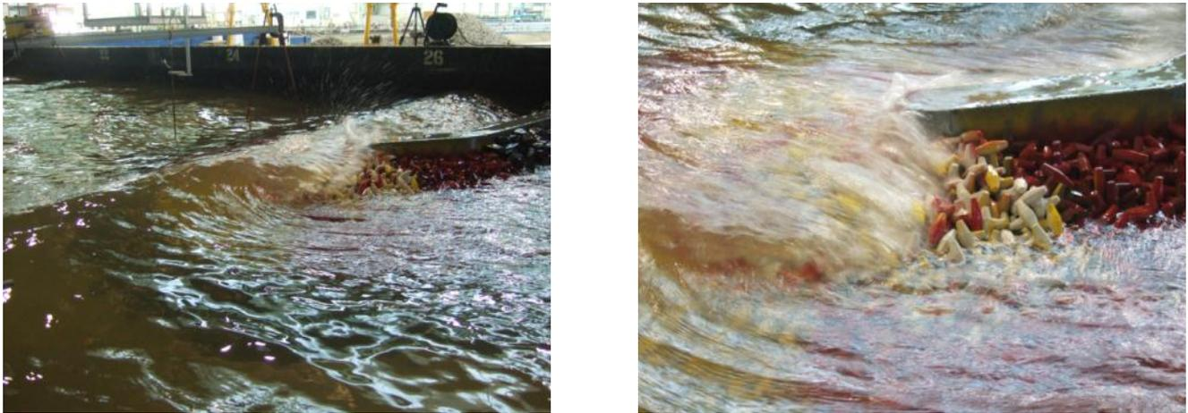
Figure 8.14 – Images of the roundhead with Core-loc during test RB-A3
