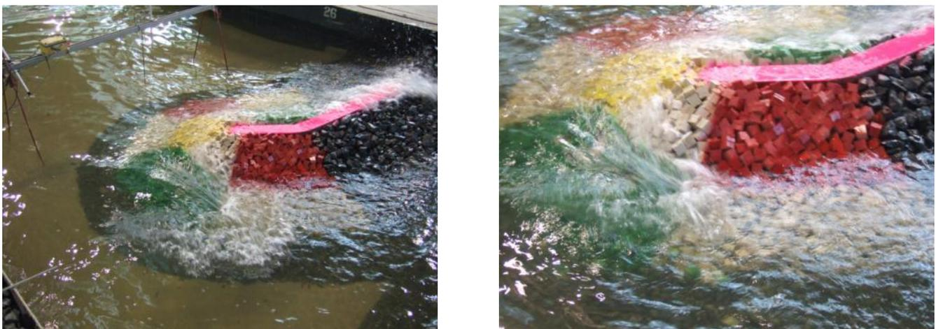
Figure 8.21 – Images of the roundhead with antifer cubes during test RB-A2
