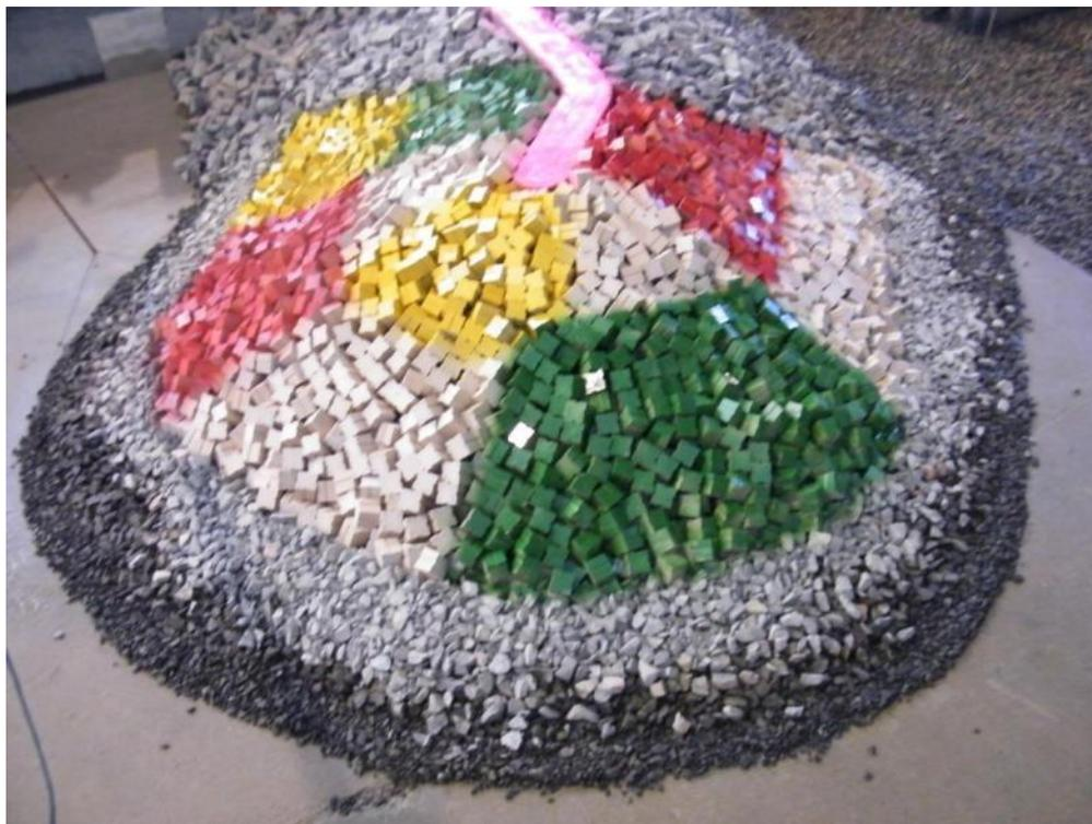
Figure 7.4 – Roundhead model of the covering alternative with 44-tonne Antifer cubes
