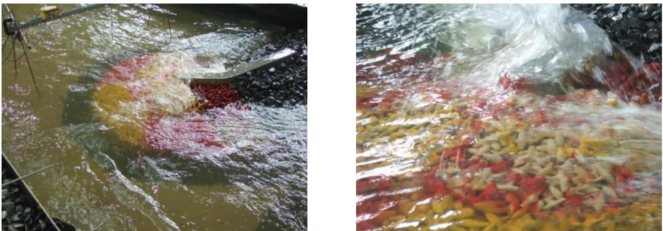
Figure 8.15 – Images of the roundhead with Core-loc during test RB-B4
