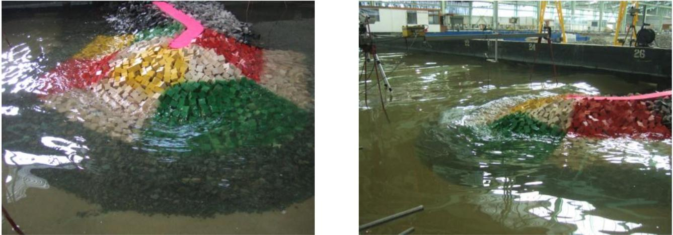
Figure 8.18 – Images of the roundhead with antifer cubes during test RB-B1
