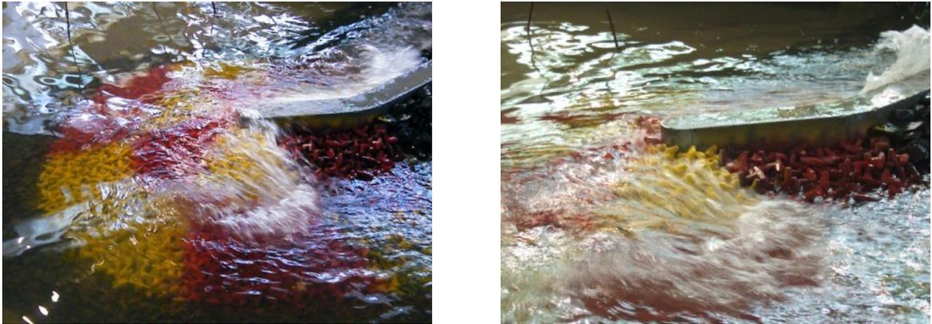
Figure 8.12 – Images of the roundhead with Core-loc during test RB-A2
