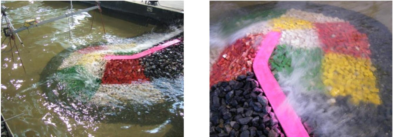
Figure 8.20 – Images of the roundhead with antifer cubes during test RB-B2
