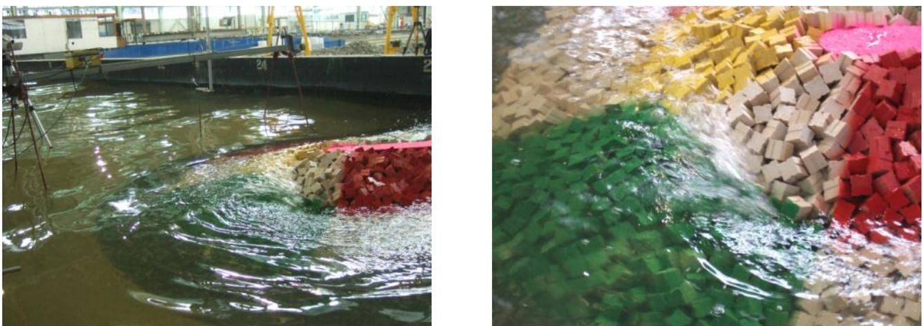
Figure 8.19 – Images of the roundhead with antifer cubes during test RB-A1
