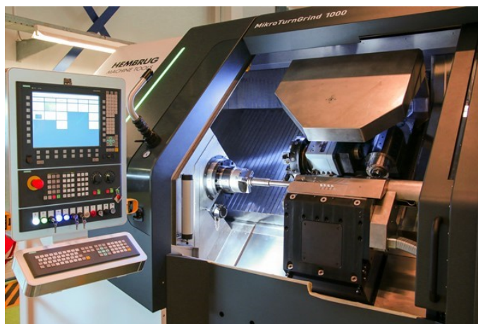
Figure 1.1: A general overview of a horizontal turning machine from the company Hembrug.
