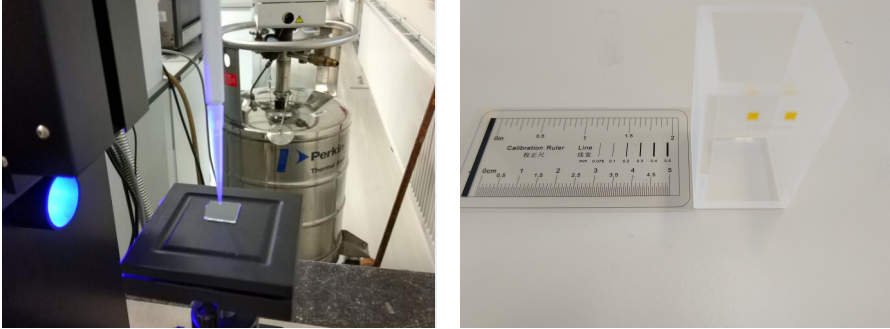
(a) The pipette tip of the CAM 200 instrument is placing one droplet of water on the surface of one piece of glass.
