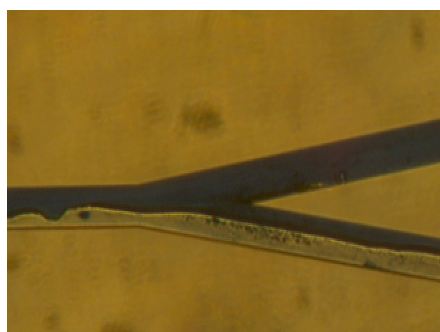
(a) Leakage of water to the toluene outlet. The Ca number of toluene is 2.18 \times 10^{-3} . The volumetric flow rate ratio ( \Phi_{aq}/\Phi_{org} ) of these two phases is 0.8.
