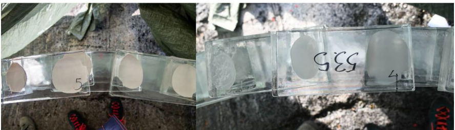
9. Top view of bonded bricks with the Fast-curing experimental Dowsil Adhesive (left) and 3M DP610 (right).
