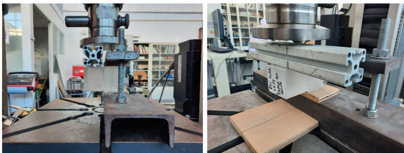
Fig. 10 Experimental set-up of the shear tests
