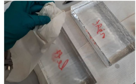
6. Bricks are removed and cleaned using isopropanol
