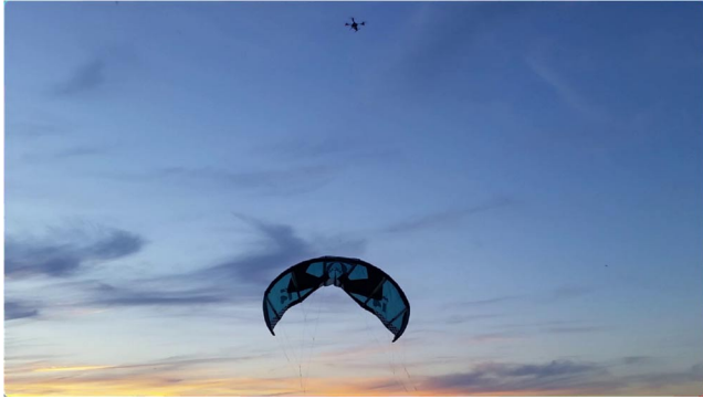
Fig. 1 Custom-made drone launching a 9 m 2 kite. Photo credit: Marcos Jerez Venegas.
