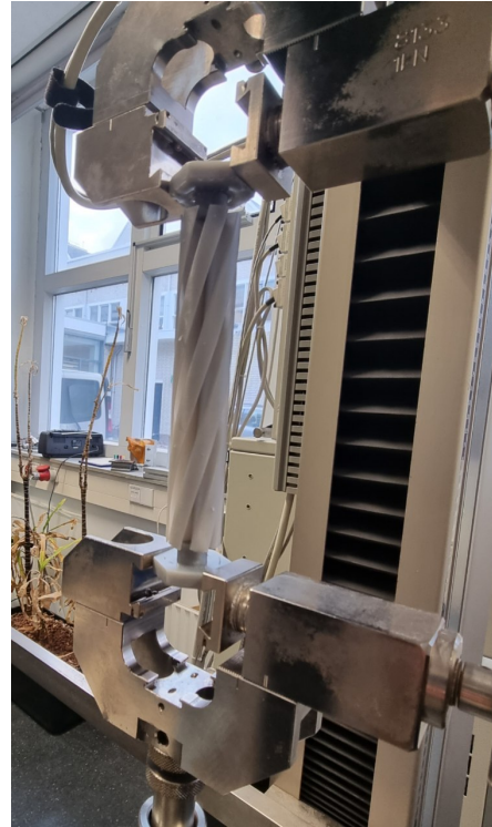
Figure 2.6.: 3D-printed prototype and the test setup
