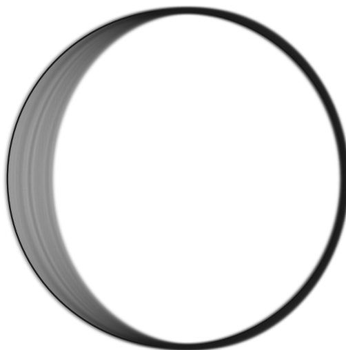
Figure 3.3: An extreme example of a blob forming along the contour of a sphere for the left viewpoint when drawing the whole path naively.
