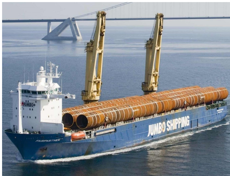
Figure 1.1: Jumbo Maritime's J-type vessel the "Fairpartner" carrying large monopiles for the Yunlin project
