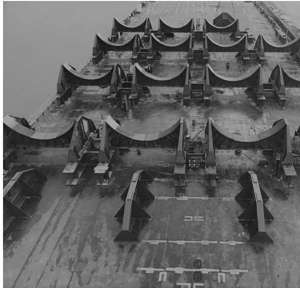
Figure 2.2: General saddle orientation on the top deck
