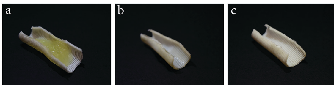
Fig. 10 Coagulation of human plasma in circulating model. The PTFE vein implant untreated (a), coated with SK@alumina (b), or coated with the Hep_MIL-101(Fe) + SK@alumina hybrid (c).
