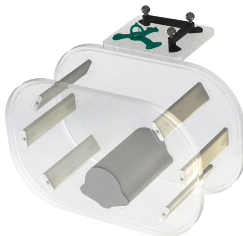
Figure A.3. Structural design of the customized abdominal phantom, including six ribs, a spine enclosed between two plexiglass plates and a platform containing both an EM active tracker and an optical fiducial tracker.
