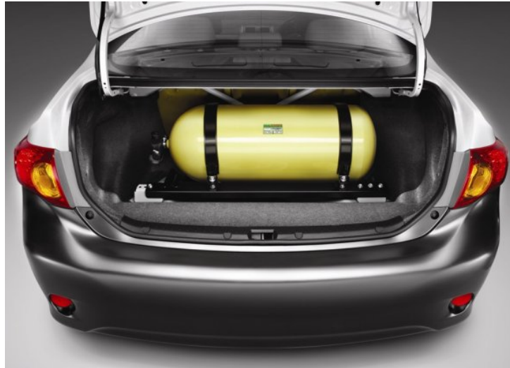
Figure 1.1: Typical size and position of a pressurized CNG tank, from NGV Depot [2018]
