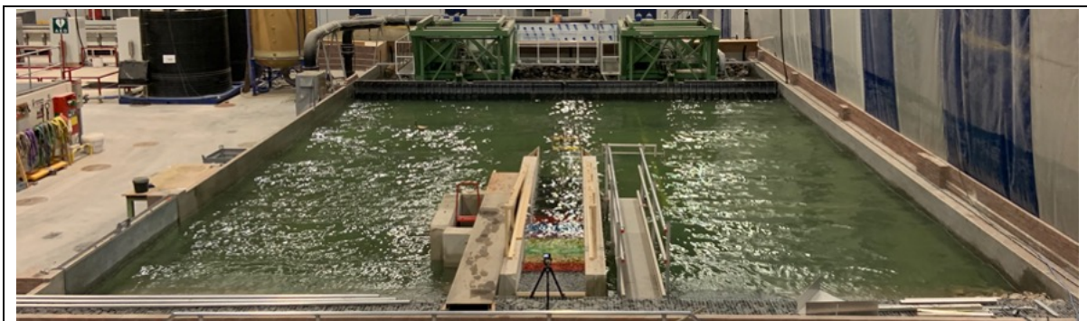
Figure 13: The Pacific basin facility at Deltares during a test. The flume with the mild slope can be seen in the middle.
