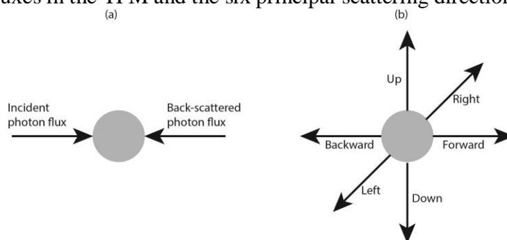
**Figure 7: Schematic representation of (a) photon fluxes in the Two-Flux Model; (b) the six principal directions of photon scattering in the Six-Flux Model. (after [85])**
