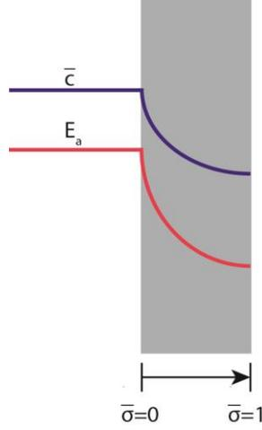
**Figure 8: Schematic of the dimensionless concentration profile and the dimensionless rate of photon absorption along a 1D slab**
