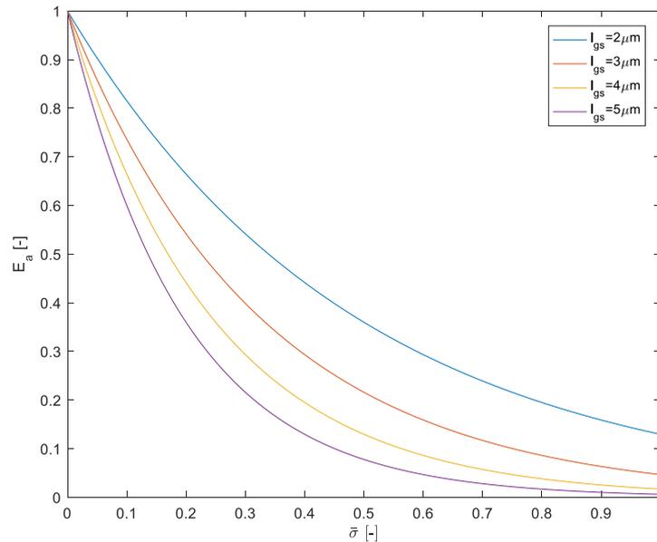
**Figure 10: Dimensionless photon flux along the photocatalytic film thickness for different film thickness**
