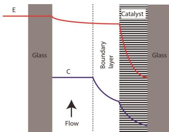
Figure 6: Schematic representation of the radiation and pollutant concentration profile in the flat-plate photocatalytic reactor considering external mass transfer limitations and light absorption by the flow (after [72]).
