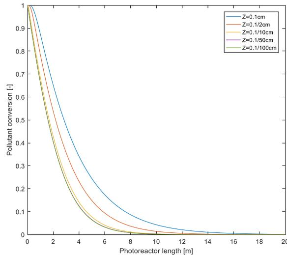
**Figure 15: Limiting case of the pollutant conversion at different photoreactor heights**
