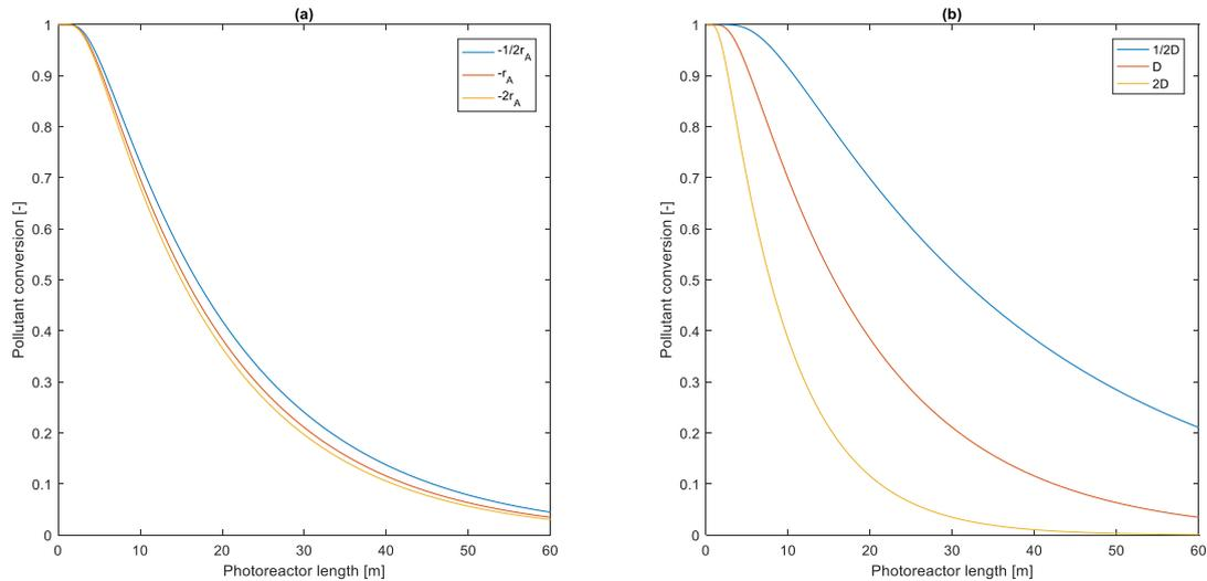
**Figure 13: Outline of the pollutant conversion at the top area of the reactor along the reactor length for (a) different values of reaction rates, and (b) different values of the diffusion coefficient**
