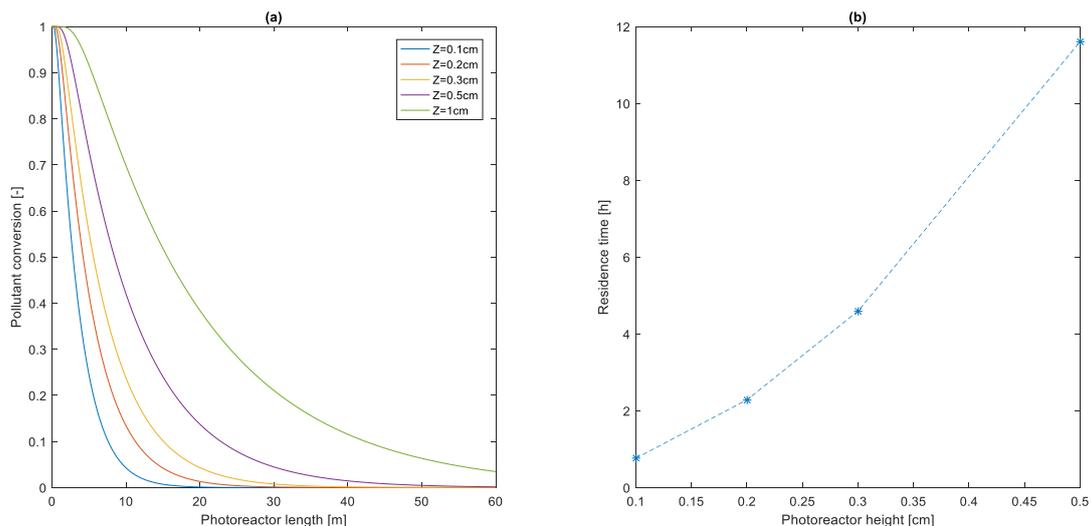
**Figure 14: (a) Pollutant conversion varying the photoreactor height; (b) Residence time to achieve 95% conversion for different photoreactor height**
