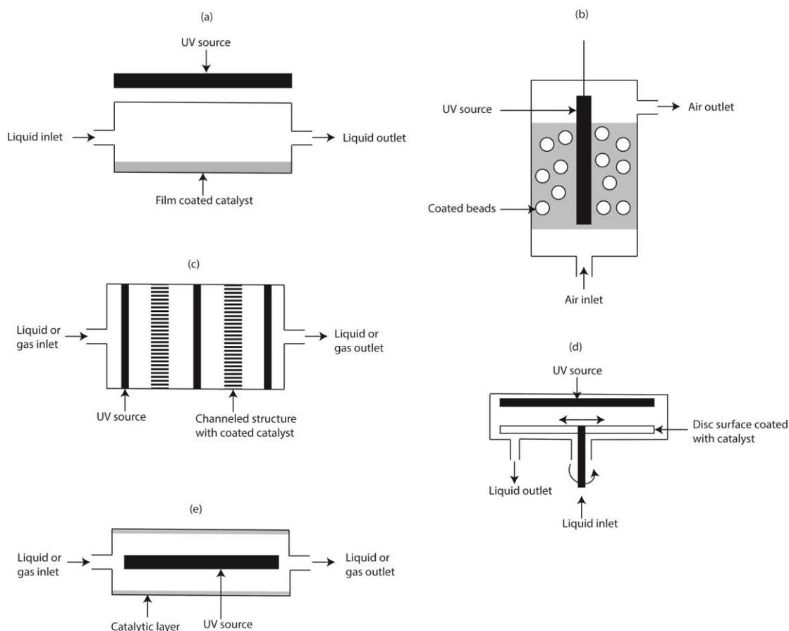
**Figure 4: Examples of different photoreactors: (a) Flat-plate with immobilized catalyst photoreactor (after [50]), (b) Slurry fluidized bed photoreactor (after [51]), (c) Monolith photoreactor (after [52]), (d) Spinning disc photoreactor (after [53]), (e) Annular photoreactor (after [54]).**
