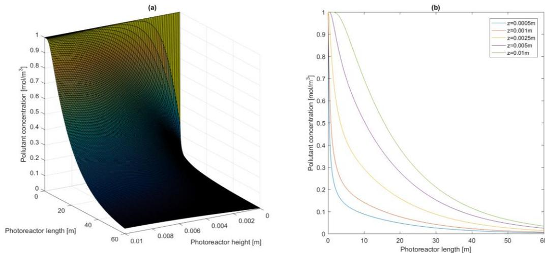
**Figure 12: (a) Outline of the pollutant concentration along the photoreactor; (b) Pollutant concentration profile along the photoreactor length at different photoreactor heights,  $z$ .**
