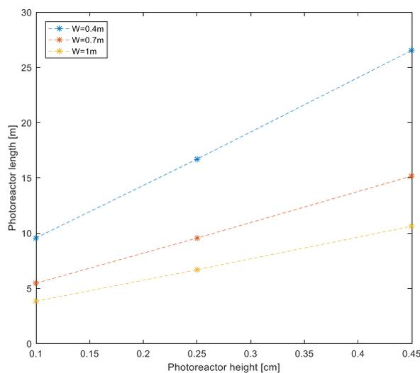
**Figure 16: Photoreactor length to reach 95% conversion for different photoreactor height and width**
