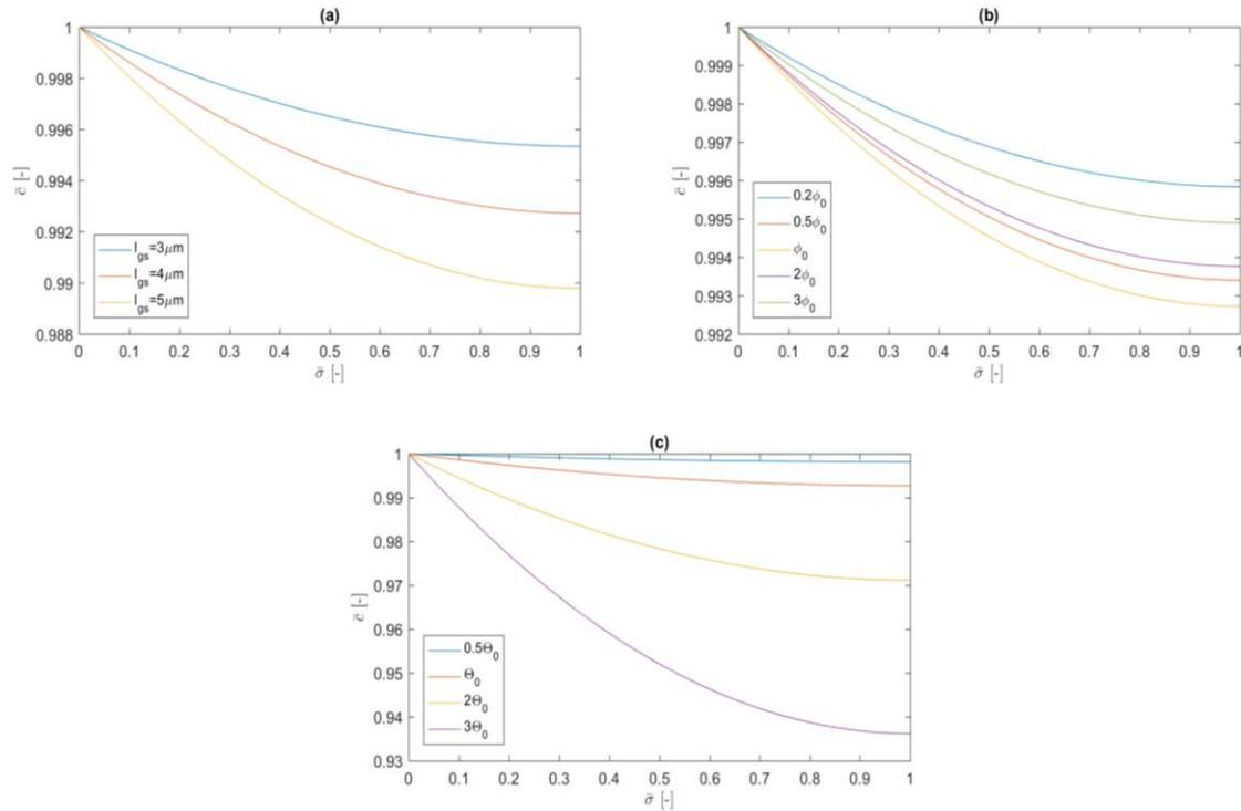
**Figure 11: Dimensionless concentration profile along the catalyst film thickness for (a) different catalyst thickness; (b) different equilibrium adsorption constant for a catalyst thickness of 4 $\mu\text{m}$ ; (c) different Thiele modulus for a catalyst thickness of 4 $\mu\text{m}$ .**
