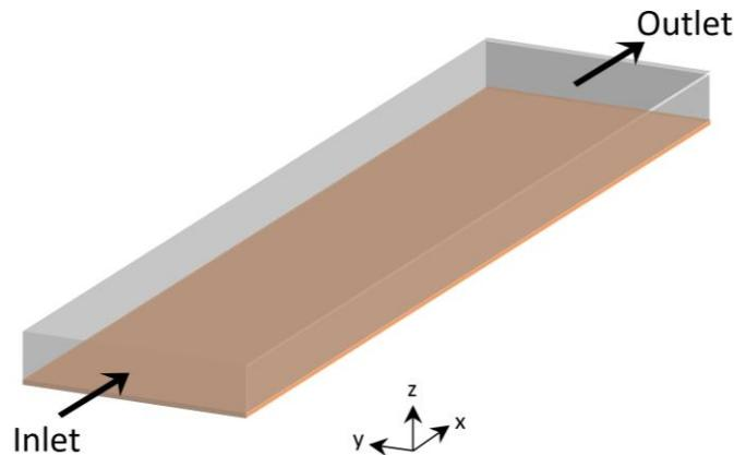
**Figure 9: 3D view of the flat plate photoreactor with the film photocatalyst deposited at the bottom**
